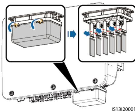
**Step 2** Connect the AC output power cable.
