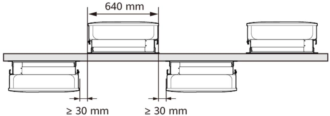
**Figure 4-9** Support-mounted dual-track back-to-back installation (not recommended)
