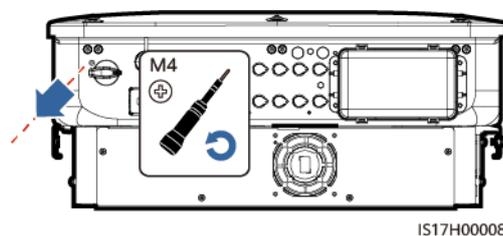
**Step 3** Turn on the DC switch at the bottom of the SUN2000.
