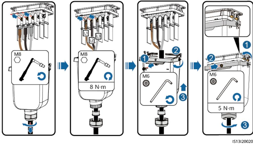
Figure 5-11 Wiring requirements
