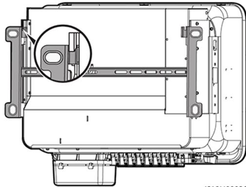
**Step 3** Tighten the nuts on both sides of the SUN2000.
