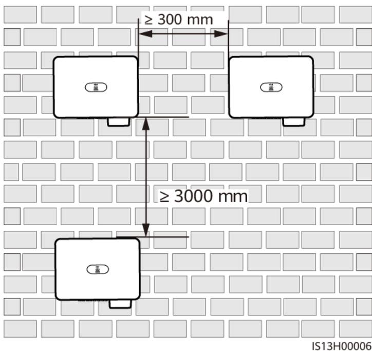
**Figure 4-7** Support-mounted dual-track spaced installation (recommended)
