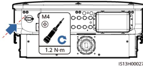
**Step 5** Turn off the DC switch (if any) between the SUN2000 and PV strings.
