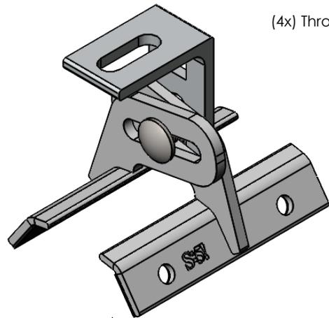
(4x) Through hole for fasteners
