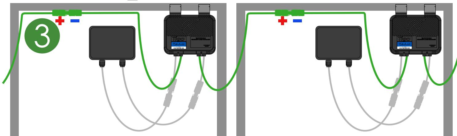
Note: When installing TS4-A or TS4-A-Duo, connect the input cables to the PV module before connecting the TS4-A output cables in series.
