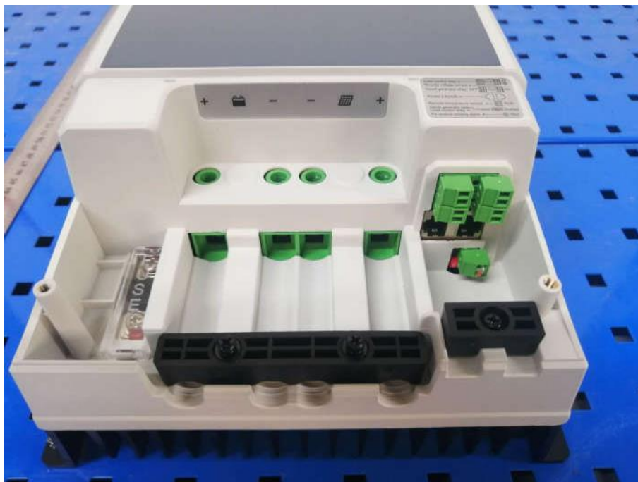
Fig3 Internal terminal identification of the BCC--Tracer10420AN
