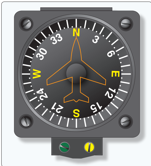
Figure 10-81. A vertical magnetic direction indicator provides a realistic reference of headings.
