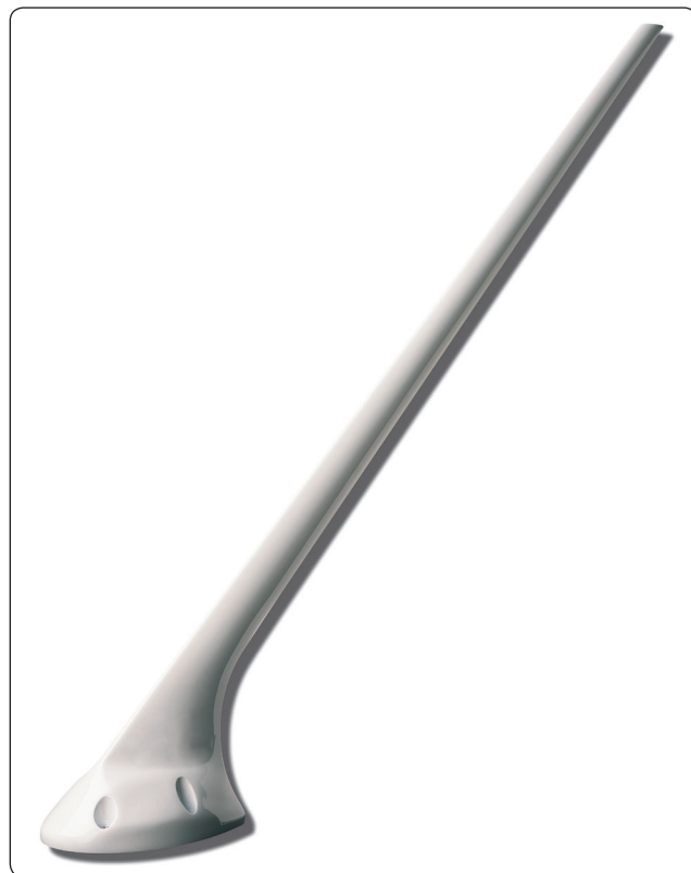
Figure 11-90. Many antenna are canted for better reception.
