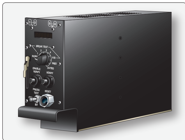
Figure 13-108. A rack mounted antiskid control unit from an airliner.
