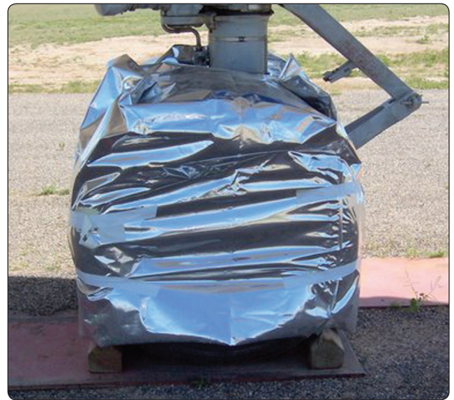
Figure 13-145. Cover tires to protect from harmful chemicals and from the elements when parked outside for long periods of time.
