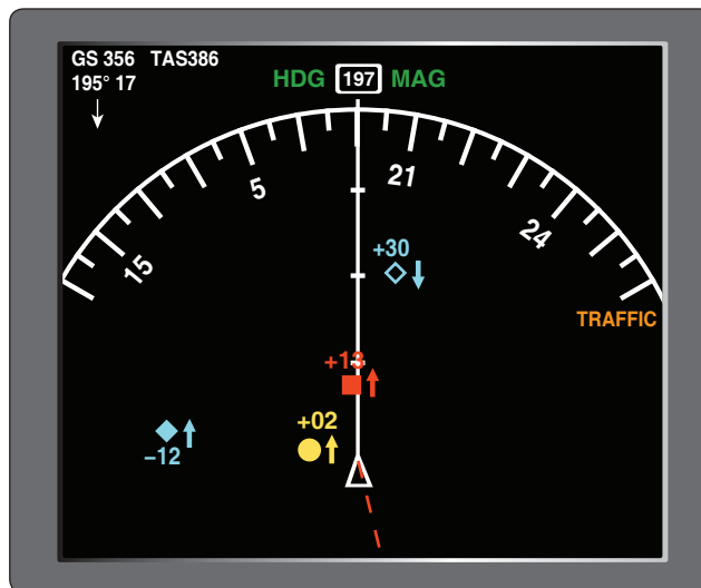
Figure 11-133. TCAS information displayed on a multifunction display. An open diamond indicates a target; a solid diamond represents a target that is within 6 nautical miles of 1,200 feet vertically. A yellow circle represents a target that generates a TA (25-48 seconds before contact). A red square indicates a target that generates an RA in TCAS II (contact within 35 seconds). A (+) indicates the target aircraft is above and a (-) indicates it is below. The arrows show if the target is climbing or descending.
