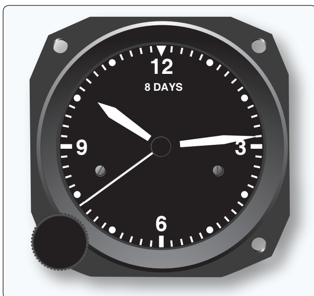
Figure 10-131. A typical mechanical 8-day aircraft clock.
