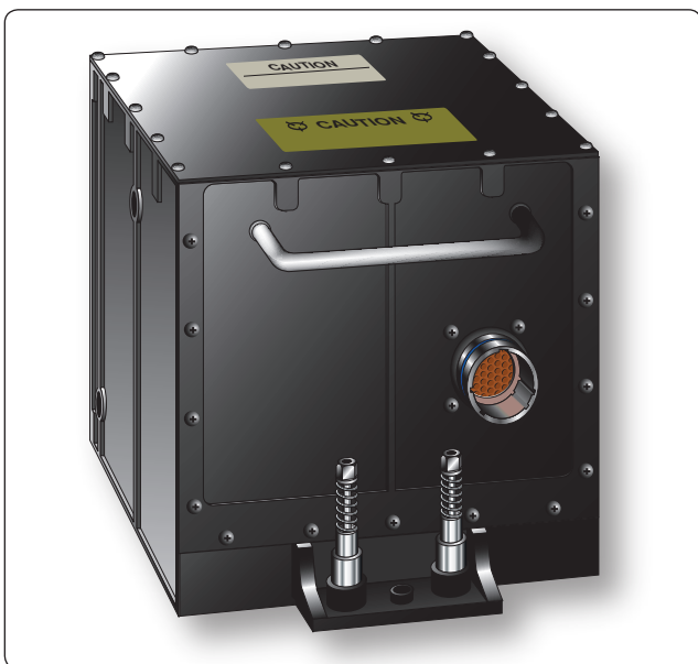
Figure 11-156. A modern micro-IRS with built-in GPS.
