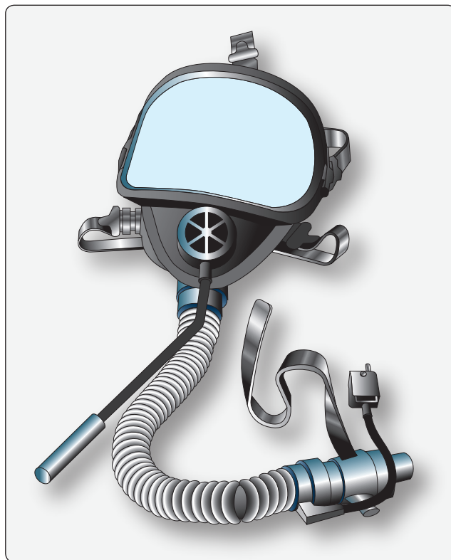
Figure 16-33. Smoke masks cover the eyes as well as the nose and mouth of the user.
