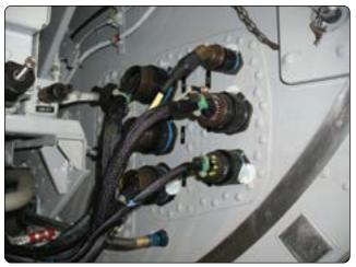
Figure 9-158. Electrical connectors.
