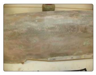
Figure 7-8. Copper mesh lightning protection material.
