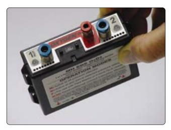
**Figure 16-24.** A portable two-person electronic pulse-demand (EPD) oxygen regulating unit.
