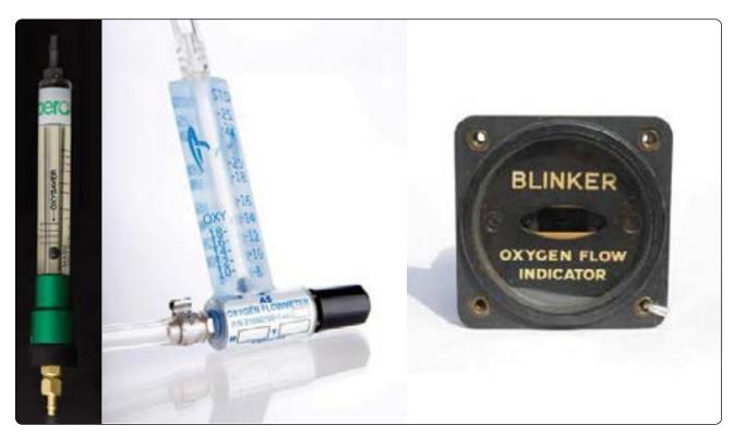
**Figure 16-23.** Different flow indicators are used to provide verification that the oxygen system is functioning: continuous-flow, inline (left); continuous-flow, inline with valve adjuster (center); and old style demand flow (right).
