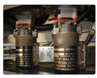
Figure 12-48. Shutoff valves.
