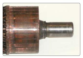
Figure 9-44. Typical DC generator commutator.
