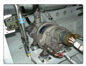
Figure 12-22. *Electrically-driven pump*.
