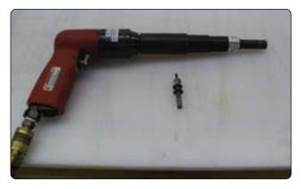
Figure 4-112. Drive nut blind bolt installation tool.
