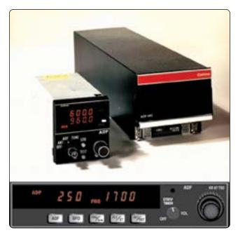
**Figure 11-107.** A flight deck mountable ADF receiver used on general aviation aircraft.
