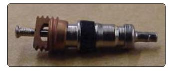
**Figure 13-149.** The tire valve core should be removed after the tire is completely deflated and before the tire and wheel assembly is removed from the aircraft.
