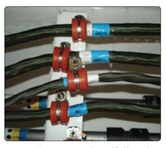
**Figure 9-133.** Positive separation of wire and fluid lines and wire clamps.
