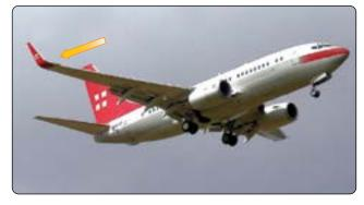
**Figure 1-77.** A winglet reduces aerodynamic drag caused by air spilling off of the wing tip.
