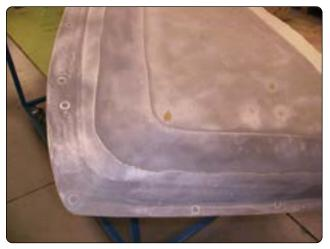
Figure 7-9. Aluminum mesh lightning protection material.
