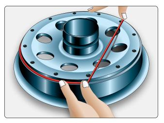
**Figure 13-154.** The wheel half O-ring for a tubeless tire wheel assembly must be in good condition and lubricated to seal for the entire life of the tire. The mating surfaces of the wheel halves must also be in good condition.
