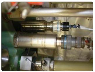
Figure 12-11. Temperature and quantity sensors.
