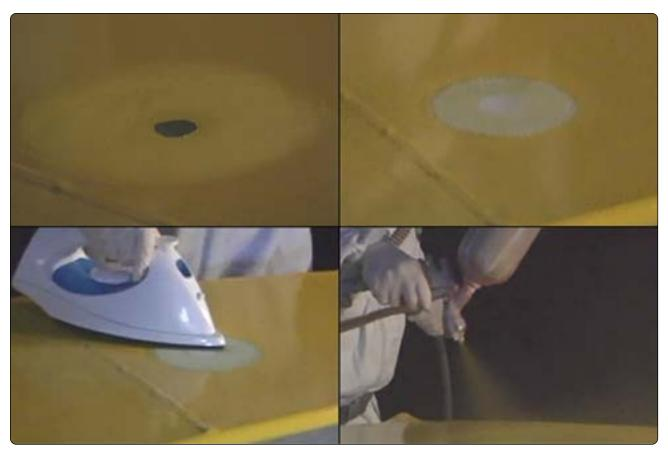
**Figure 3-36.** A patch over this small hole on a polyurethane top coat is repaired in accordance with the repair instructions in the STC under which the aircraft was re-covered. It requires only a two-inch fabric overlap and scuffing into the top coat before cementing and refinishing. Other STC repair instructions may not allow this repair.
