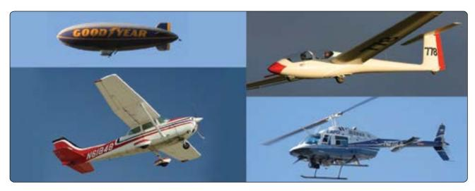
Figure 1-11. Examples of different categories of aircraft, clockwise from top left: lighter-than-air, glider, rotorcraft, and airplane.
