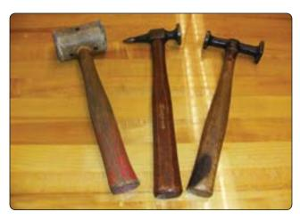
Figure 4-69. Sheet metal mallet and hammers.
