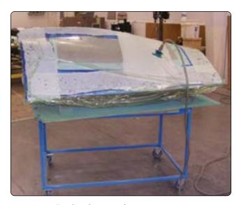
Figure 7-52. Envelope bagging of repair.
