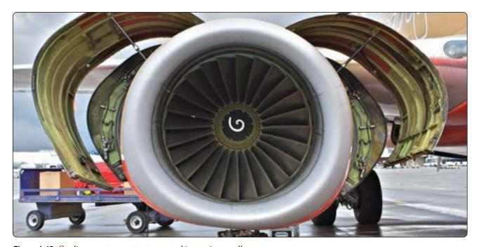
**Figure 1-45.** Cowling on a transport category turbine engine nacelle.
