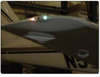
**Figure 9-175.** A right wing tip position light, also known as a navigation light.
