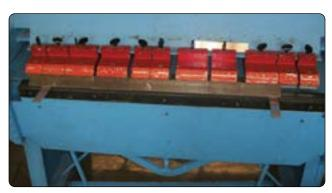
**Figure 4-142.** Brake alignment with two test strips 3 inches from each end.
