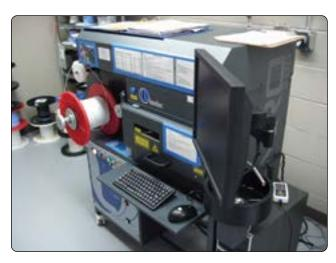
Figure 9-126. Laser wire printer.
