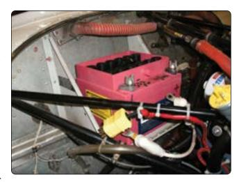
Figure 9-32. Lead-acid battery installation.
