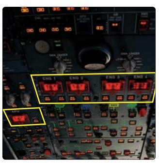
**Figure 17-16.** Engine and APU fire switches on the flight deck center overhead panel.
