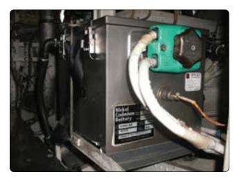
Figure 9-34. NiCd battery installation.
