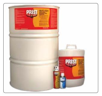
**Figure 14-9.** Fuel anti-icing products, such as  $Prist^{\circledast}$ , act as antifreeze for any free water in aircraft fuel. They dissolve in the water and lower its freezing point to prevent ice crystals from disrupting fuel flow.
