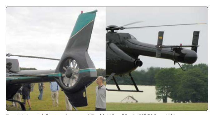
Figure 2-28. Aerospatiale Fenestron tail rotor system (left) and the McDonnell Douglas NOTAR® System (right).
