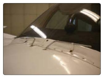
Figure 15-46. Chemical deicing spray tubes.
