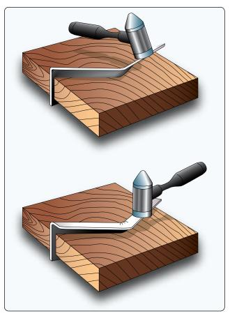
Figure 4-153. Stretching a flanged angle.
