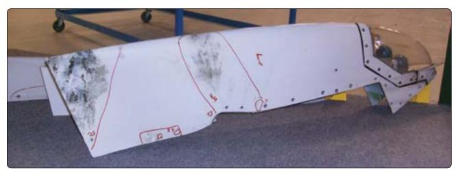
Figure 7-22. Erosion damage to wingtip.
