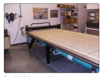
Figure 7-89. Gerber cutting table.
