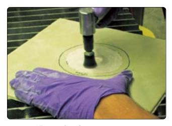
Figure 7-58. Taper sanding of repair area.
