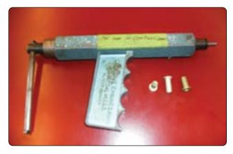
Figure 4-113. Rivet nut installation.
