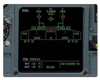
Figure 14-39. The graphic depiction of the fuel system on this electronic centralized aircraft monitor (ECAM) fuel page includes valve position information.
