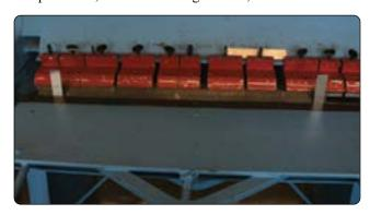
**Figure 4-143.** *Brake alignment with two test strips bent at* 90°.
