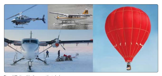
**Figure 1-83.** Aircraft landing gear without wheels.
