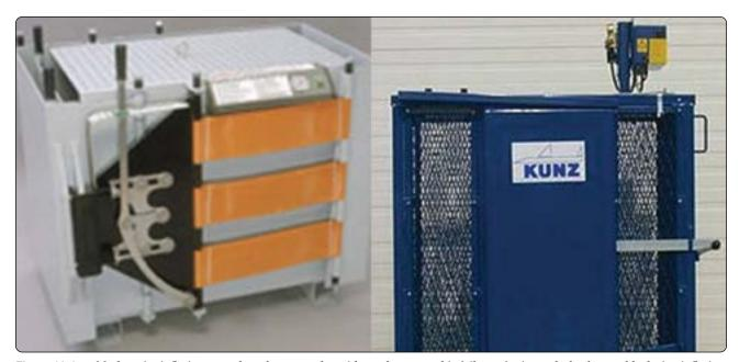
**Figure 13-155.** Modern tire inflation cages have been tested to withstand catastrophic failure of a tire and wheel assembly during inflation. All newly mounted tires should be inflated in such a cage.
