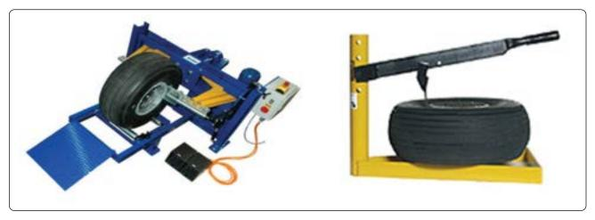
Figure 13-151. An electrohydraulic tire bead breaker (left) used on large tires and a manual tire bead breaker (right) used on small tires.
