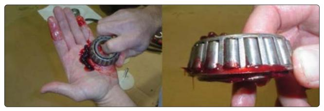
**Figure 13-46.** Packing grease into a clean, dry bearing can be done by hand in the absence of a bearing grease tool. Press the bearing into the grease on the palm of the hand until it passes completely through the gap between the rollers and the inner race all the way around the bearing.
