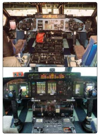
**Figure 10-2.** A conventional instrument panel of the C-5A Galaxy (top) and the glass flight deck of the C-5B Galaxy (bottom).
