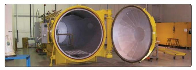
Figure 7-39. Autoclave.
