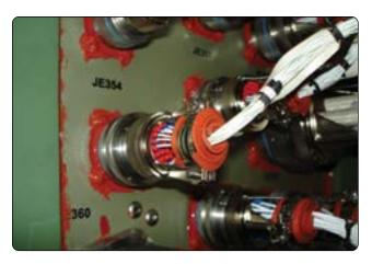
Figure 9-162. Backshells with strain relief.
