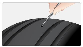
Figure 13-139. Deflate a tire before removing or probing any area where a foreign object is lodged.
