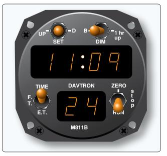
Figure 10-132. A typical aircraft electronic clock.
