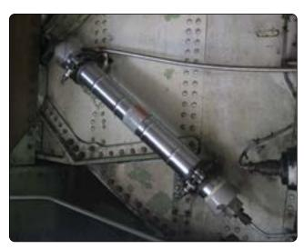
Figure 12-50. Cylindrical accumulator.
