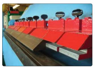
Figure 4-135. Brake radius nosepiece adjustment.
