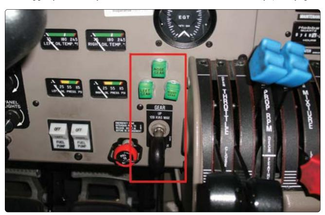
Figure 9-94. Instrument panel showing the landing gear position switch and the three gear down indicators.
