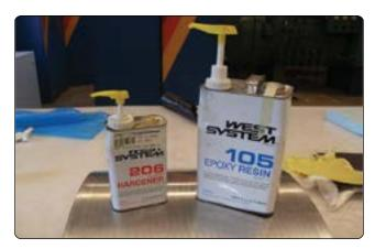
**Figure 7-10.** Two-part wet layup epoxy resin system with pump dispenser.
