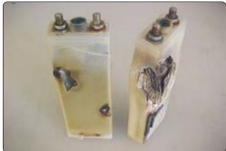
Figure 9-35. Thermal runaway damage.
