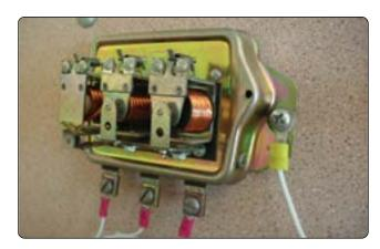
**Figure 9-59.** The three relays found on this regulator are used to regulate voltage, limit current, and prevent reverse current flow.
