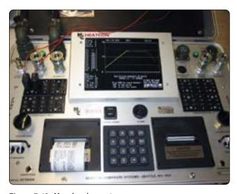
Figure 7-40. Heat bonder equipment.
