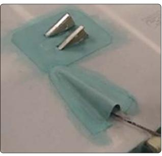
**Figure 3-33.** A strut fitting and cable guide with reinforcing fabric gussets cemented in place.
