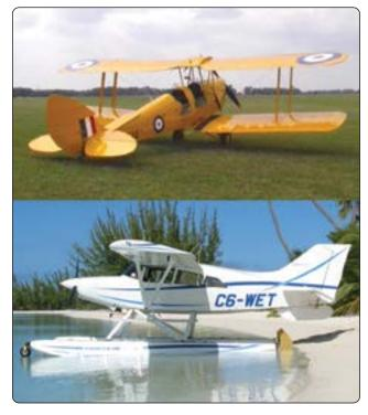
Figure 3-1. Examples of aircraft produced using fabric skin.
