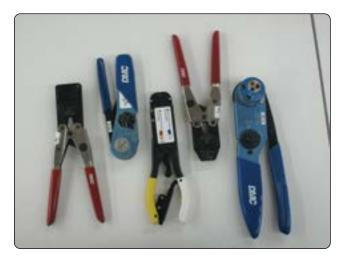
Figure 9-156. Crimping pliers.
