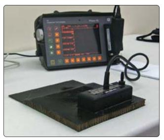
Figure 7-28. Phased array testing equipment.
