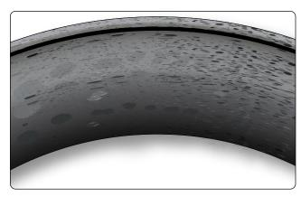
Figure 13-72. Bruising is caused by fine particle contamination possibly from a bad seal or improper maintenance of bearing cleanliness. It leaves a less than smooth surface on the bearing cup.
