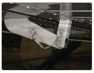
Figure 9-145. Bonding jumpers.
