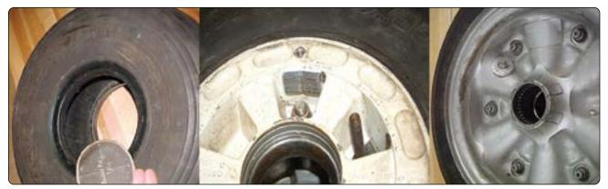
Figure 13-160. A tire balancing patch (left), adhesive wheel weights (center), and a bolted wheel weight (right) are all used to balance aircraft tire and wheel assemblies per the manufacturer's instructions.
