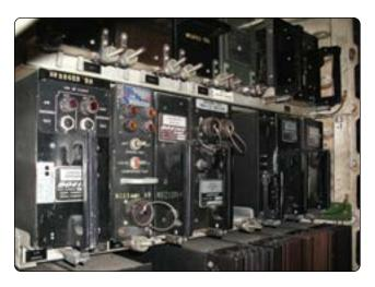
Figure 9-81. Line replaceable units in an equipment rack.
