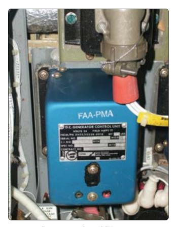
Figure 9-56. Generator control unit (GCU).
