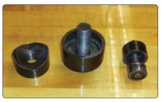
Figure 4-14. Chassis punch.
