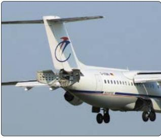
Figure 2-16. Speed brake.
