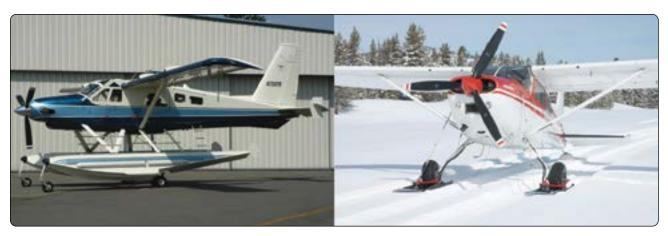
Figure 13-2. An amphibious aircraft with retractable wheels (left) and an aircraft with retractable skis (right).
