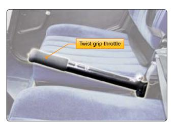
**Figure 2-46.** A twist grip throttle is usually mounted on the end of the collective lever. The throttles on some turbine helicopters are mounted on the overhead panel or on the floor in the flight deck.
