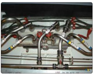
Figure 12-35. Four-way servo control valve.
