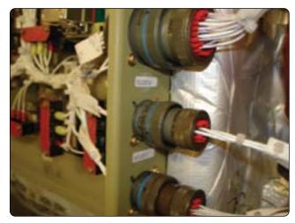
Figure 9-161. Connector arrangement to avoid wrong connection.
