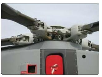
**Figure 1-99.** Five-blade articulated main rotor with elastomeric bearings.
