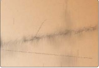
Figure 8-19. Example of sanding scratches.
