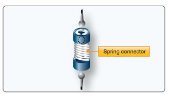
Figure 2-78. Spring-type connector.
