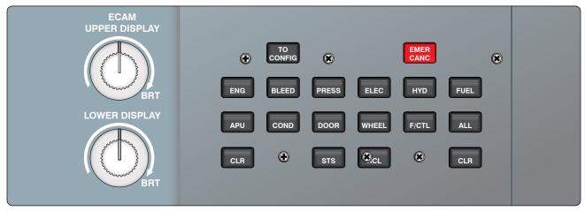
Figure 10-121. An ECAM display control panel.
