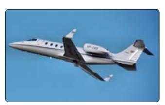
Figure 2-17. Winglets on a Bombardier Learjet 60.
