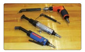
Figure 4-40. Angle drill motors.
