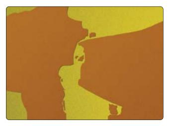
Figure 8-13. Example of poor adhesion.
