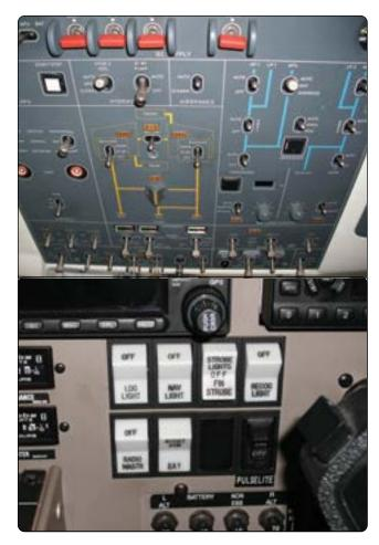
Figure 9-167. Toggle and rocker switches.
