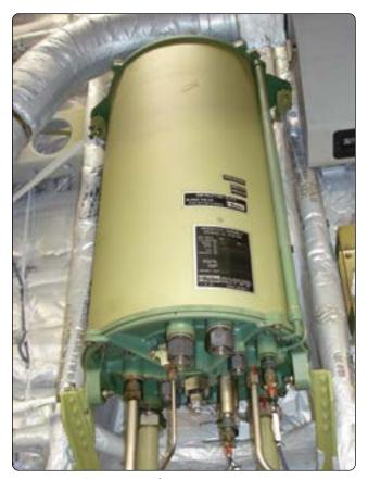
Figure 12-9. Air-pressurized reservoir.
