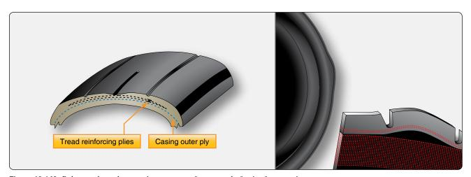
**Figure 13-142.** Bulges and tread separation are cause for removal of a tire from service.
