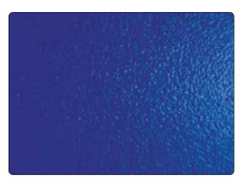
Figure 8-17. Example of orange peel.
