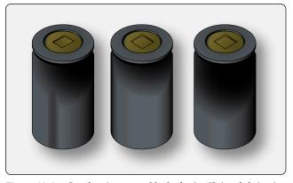
Figure 13-67. Overheating caused by lack of sufficient lubrication results in a bluish tint to the metal surface. The ends of the rollers shown were overheated causing the metal to flow and deform, as well as discolor. The bearing cup raceway is usually discolored as well.
