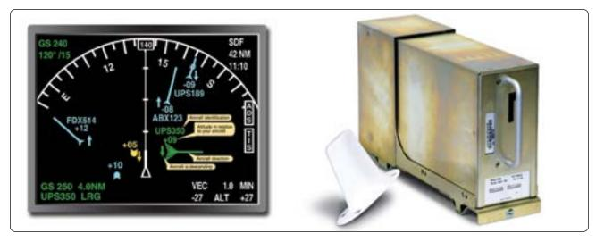
Figure 11-137. A flight deck display of ADS-B generated targets (left) and an ADS-B airborne receiver with antenna (right).
