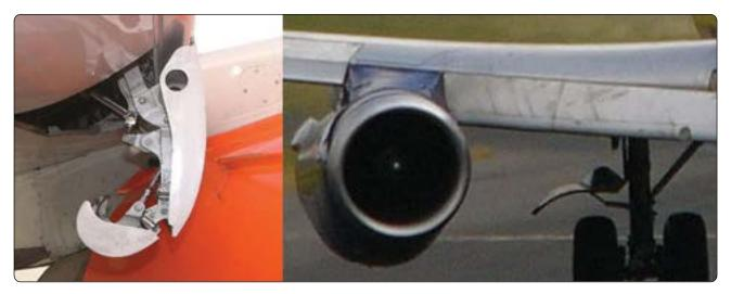
Figure 1-66. Side view (left) and front view (right) of a Krueger flap on a Boeing 737.
