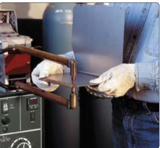
Figure 5-10. Spot welding thin sheet metal.
