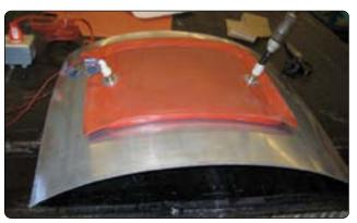
Figure 7-37. Self-sealing vacuum bag with heater element.
