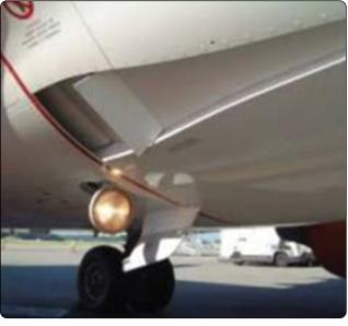
**Figure 16-66.** A ram air door controls the flow of air through the primary and secondary heat exchangers.
