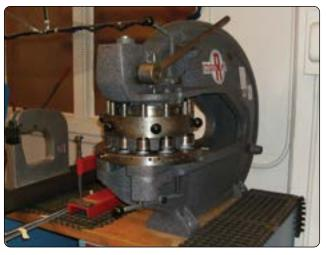
Figure 4-27. Rotary punch press.
