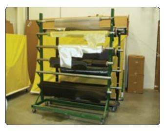
**Figure 7-12.** Dry fabric materials (top to bottom: aluminum lightning protection mess, Kevlar®, fiberglass, and carbon fiber).
