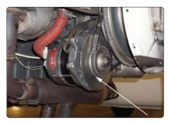
Figure 9-64. DC alternator installation.
