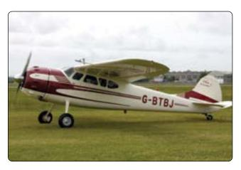
Figure 1-86. An aircraft with tail wheel gear.
