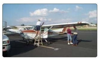
Figure 14-105. Over-the-wing refueling a Cessna.
