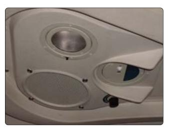
Figure 9-181. Interior flight deck and cabin light system.
