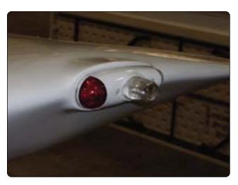
**Figure 9-174.** A left wing tip position light (red) and a white strobe light.
