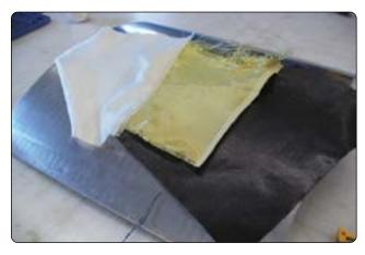
Figure 7-7. Fiberglass (left), Kevlar® (middle), and carbon fiber material (right).
