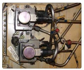
**Figure 13-112.** Two anti-skid control valves with associated plumbing and wiring.
