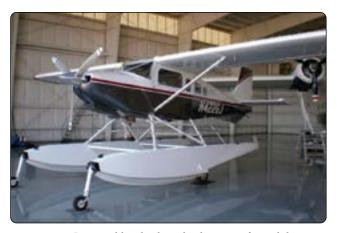
Figure 1-85. Retractable wheels make this aircraft amphibious.
