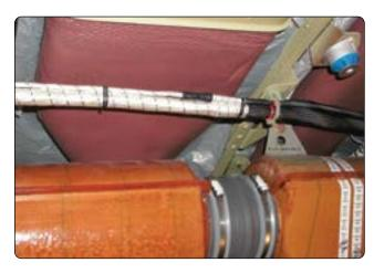
Figure 9-113. Shielded wire harness for flight control.
