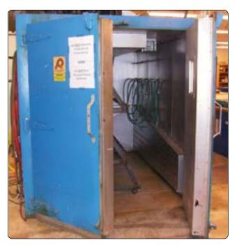
Figure 7-38. Walk-in curing oven.
