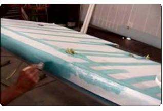
**Figure 3-34.** Cement is brushed through a four-inch tape during installation over the fabric seam on a wing leading edge. Two-inch tapes cover the wing ribs and rib lacing.
