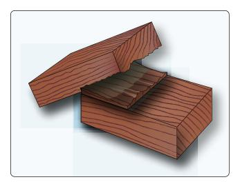
Figure 6-14. An example of good glue joint.
