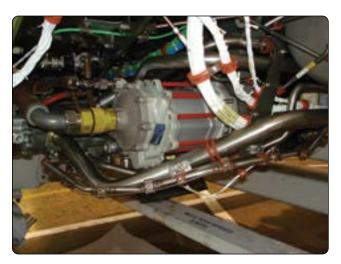
Figure 12-21. Engine-driven pump.
