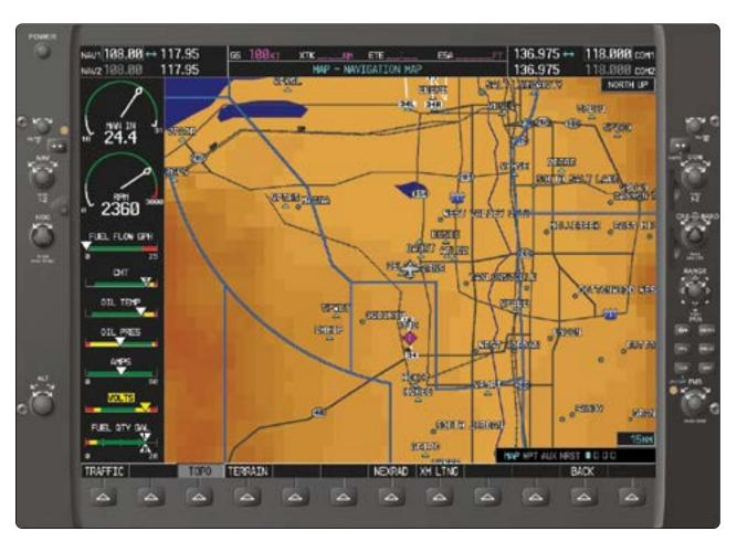
**Figure 10-14.** Oil pressure indication with other engine-related parameters shown in a column on the left side of this digital flight deck display panel.
