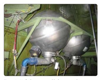
**Figure 17-12.** Built-in non-portable fire extinguisher containers (HRD bottles) on an airliner.
