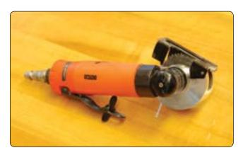
Figure 4-19. Pneumatic circular saw.
