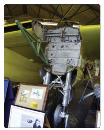
Figure 1-41. An engine nacelle firewall.
