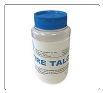
Figure 13-156. Tire talc is used on the inside of tube-type tires and the outside of aircraft tubes. This prevents binding and allows the tube to expand without stress into place within the tire.
