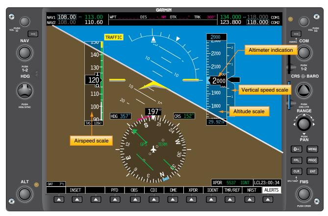
**Figure 10-34.** This primary flight display unit of a Garmin 1000 series glass flight deck instrumentation package for light aircraft indicates altitude using a vertical linear scale and a numerical counter. As the aircraft climbs or descends, the scale behind the black numerical altitude readout changes.
