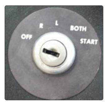
Figure 9-92. Multifunction starter switch.
