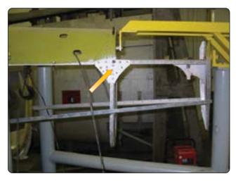
Figure 1-18. Gussets are used to increase strength.
