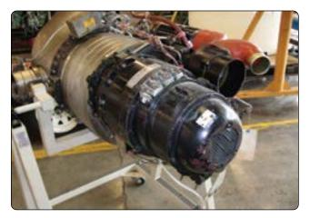
Figure 9-76. Large aircraft AC alternator.
