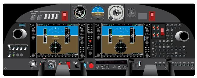
**Figure 11-70.** A modern glass flight deck on a general aviation aircraft. Digital data displays replace many older instruments and indicators of the past.
