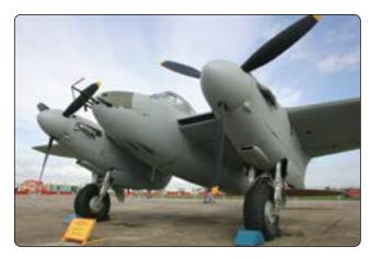
**Figure 1-9.** The De Havilland Mosquito used a laminated wood construction with a balsa wood core in the fuselage.
