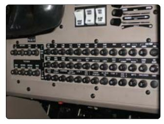
Figure 9-83. Light aircraft circuit breaker panel.
