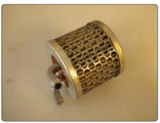
Figure 15-29. Air filter for vacuum system.
