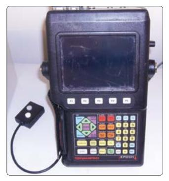
Figure 7-26. Pulse echo test equipment.
