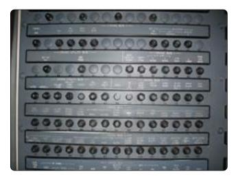
Figure 9-173. Circuit breaker panel.
