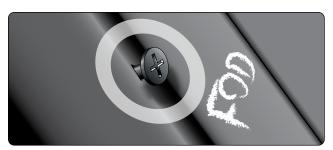
Figure 13-138. Marking of damaged area to enable closer inspection.
