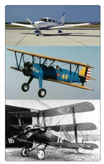
**Figure 1-12.** A monoplane (top), biplane (middle), and tri-wing aircraft (bottom).
