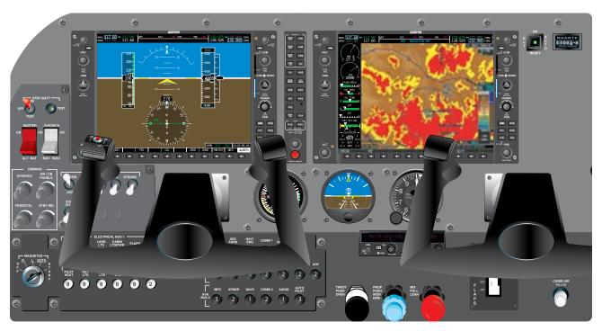
Figure 10-99. Instrumentation displayed within a glass flight deck using an attitude heading and reference system (AHRS) computer.
