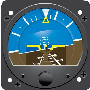
Figure 10-100. A typical vacuum-driven attitude indicator shown with the aircraft in level flight (left) and in a climbing right turn (right).
