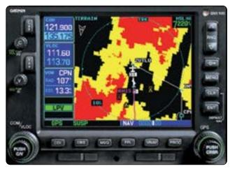
Figure 11-153. A GPS unit integrated with NAV/COM circuitry.
