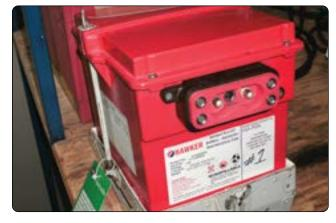
**Figure 9-33.** *Valve-regulated lead-acid battery (sealed battery).*
