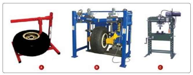
**Figure 13-64.** Tire beads must be broken from the wheel to remove the tire. A mechanical removal tool designed for breaking the bead is shown in (A); a hydraulic press designed with the capacity for large aircraft wheels is shown in (B); and an arbor press is shown in (C). All are tools available to the technician for this purpose.
