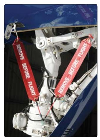
Figure 13-42. Gear pin ground lock devices.
