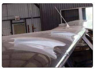
**Figure 1-79.** The Symphony SA-160 has two unique vortex generators on its wing to ensure aileron effectiveness through the stall.
