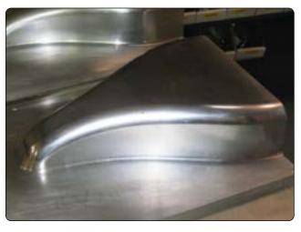
Figure 7-34. A mold of an inlet duct.
