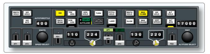
**Figure 10-112.** The AFCS control panel commands several integrated systems from a single panel including: flight directors, autopilots, autothrottles, autoland, and navigational aids. Mode selections for many features are made from this single interface.
