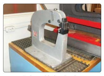
Figure 4-67. Hand-operated shrinker and stretcher unit.
