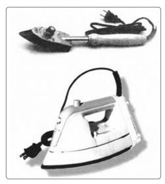
Figure 3-22. Irons used during the fabric covering process.
