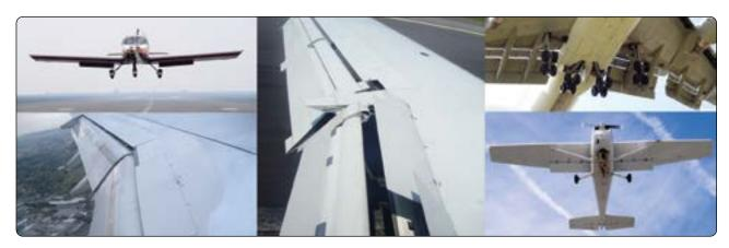
**Figure 1-62.** *Various aircraft with flaps in the extended position.*
