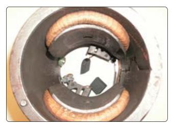
Figure 9-46. Generator field frame.
