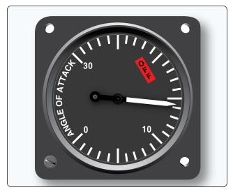
Figure 10-63. Angle of attack indicator.
