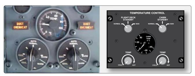
**Figure 16-70.** Typical temperature selectors on a transport category aircraft temperature control panel in the flight deck (left) and a business jet (right). On large aircraft, temperature selectors may be located on control panels located in a particular cabin air distribution zone.
