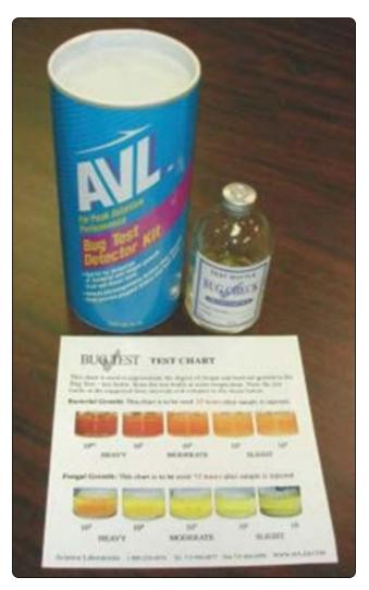
**Figure 14-100.** Fuel bug test kits identify the level of bacteria and fungus present in a fuel load by comparing the color of a treated sample with a color chart.
