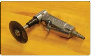
Figure 4-21. Die grinder and cut-off wheel.
