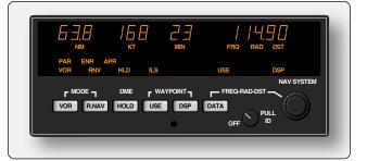
Figure 11-124. RNAV unit from a general aviation aircraft.
