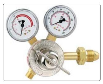
Figure 5-13. Single-stage acetylene regulator. Note the maximum 15-psi working pressure. The notched groove cylinder connection nut indicates a left-hand thread.
