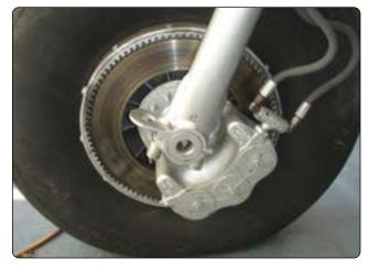
**Figure 13-79.** A single disc brake is a floating-disc, fixed caliper brake.
