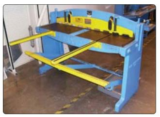
Figure 4-24. Foot-operated squaring shear.
