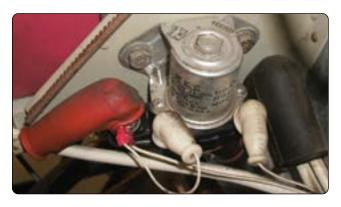
Figure 9-85. Battery solenoid.
