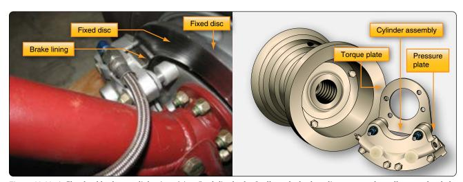
**Figure 13-82.** A Cleveland brake on a light aircraft is a fixed-disc brake. It allows the brake caliper to move laterally on anchor bolts to deliver even pressure to each side of the brake disc.
