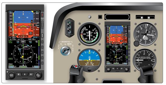
Figure 11-71. A retrofit digital data display.
