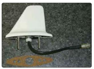
Figure 11-121. A typical aircraft-mounted DME antenna.
