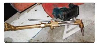
Figure 5-23. Cutting torch with additional tools.
