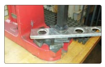
Figure 4-165. Lightening hole die set.
