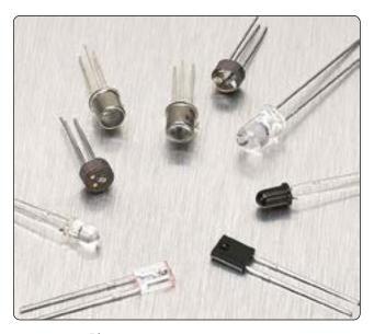
Figure 11-40. Phototransistors.
