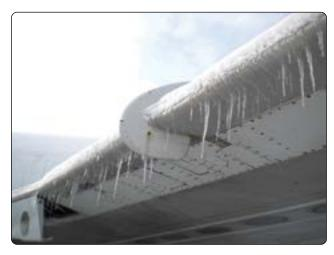
Figure 15-1. Formation of ice on aircraft leading edge.
