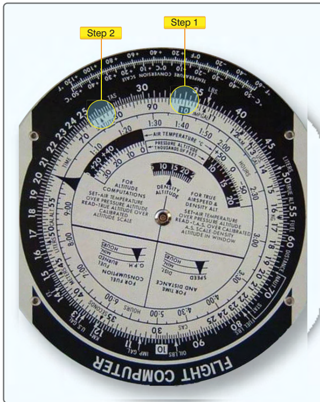
Figure 10-3. E6-B computer set up to multiply 340 by 78.
