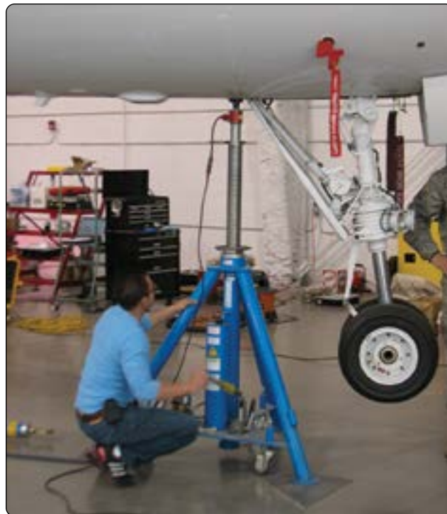
Figure 5-4. Airplane on jacks.
