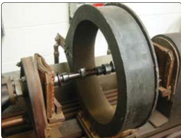
Figure 10-30. Longitudinal magnetization of camshaft (solenoid method).
