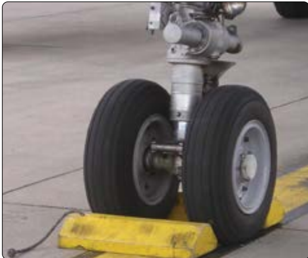
Figure 1-12. Wheels chocked fore and aft.
