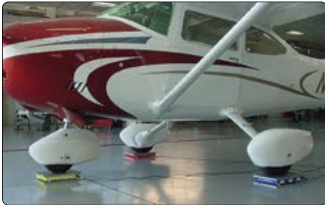
Figure 6-18. A Cessna 182 being weighed with portable electronic platform scales.
