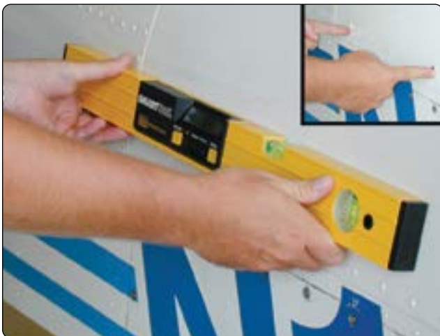
Figure 6-21. Spirit level being used on a Mooney M20.
