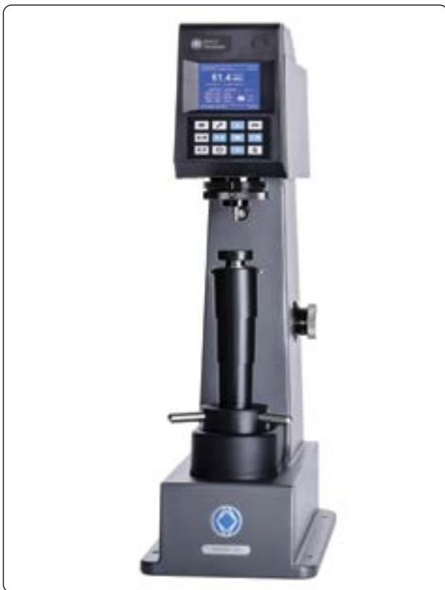
Figure 10-5. Rockwell C Hardness Tester.
