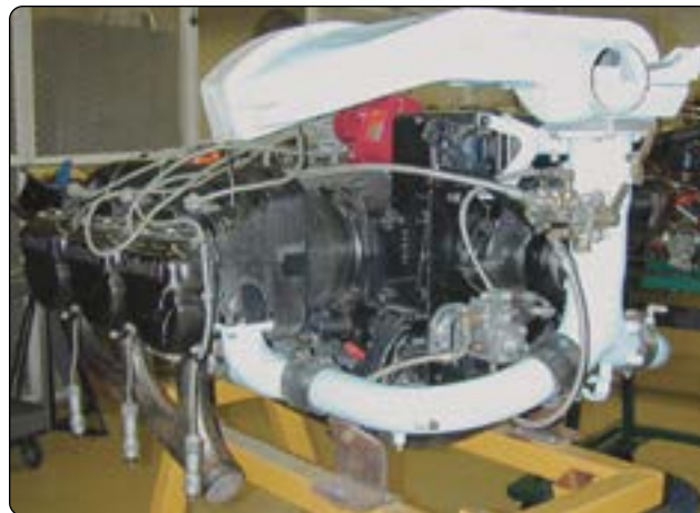
Figure 5-29. Aircraft piston engine cooled by convection.
