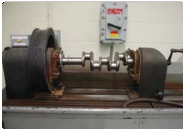
Figure 10-29. Circular magnetization of a crankshaft.
