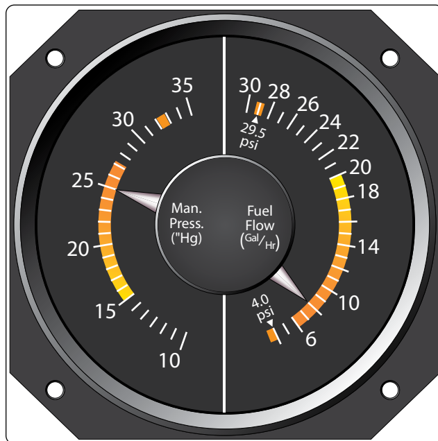
Figure 5-35. Manifold pressure gauge indicating absolute pressure.
