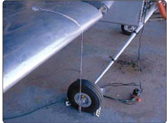
Figure 6-22. Plumb bob dropped from a wing leading edge.
