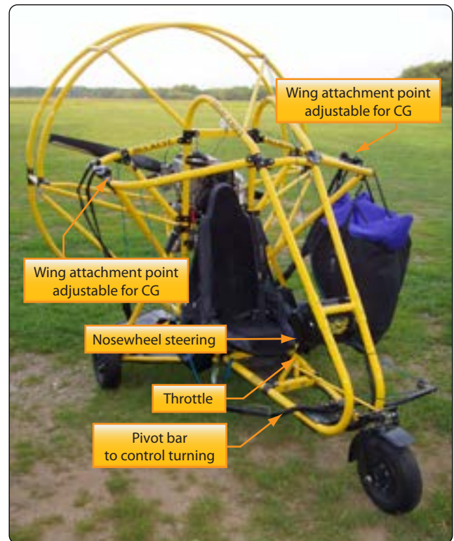
Figure 6-53. Powered parachute structure with wing attach points.
