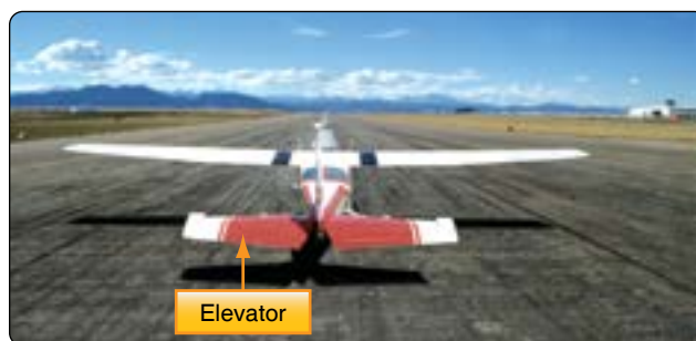
Figure 5-65. Elevator on a Cessna 182 provides pitch control.
