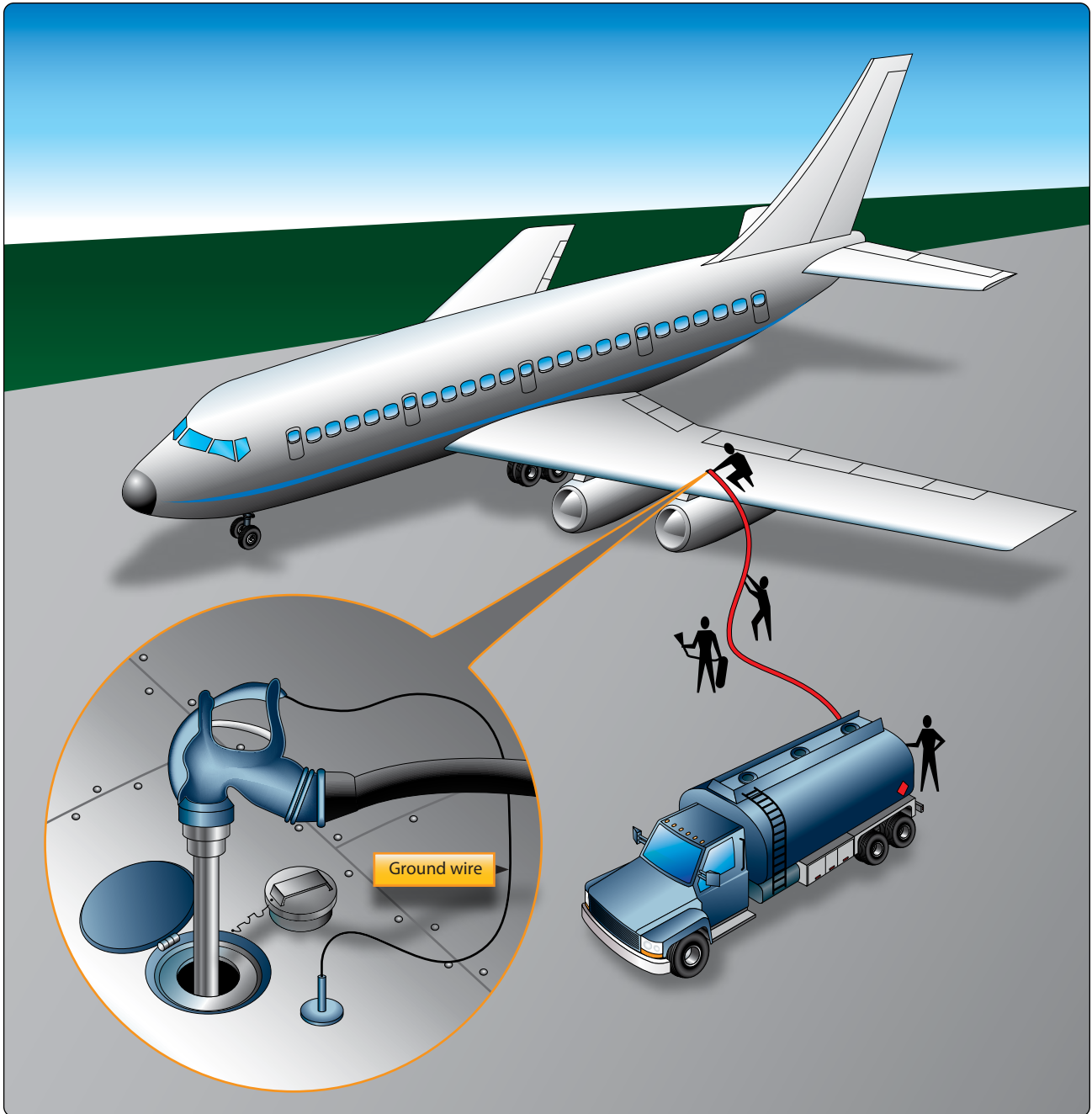
Figure 1-32. Refueling an aircraft by the over-the-wing method.
