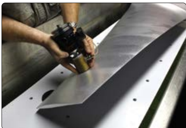
Figure 10-25. Ultrasonic inspection of a composite structure.
