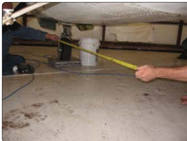
Figure 6-23. Measuring the nosewheel arm on an airplane.
