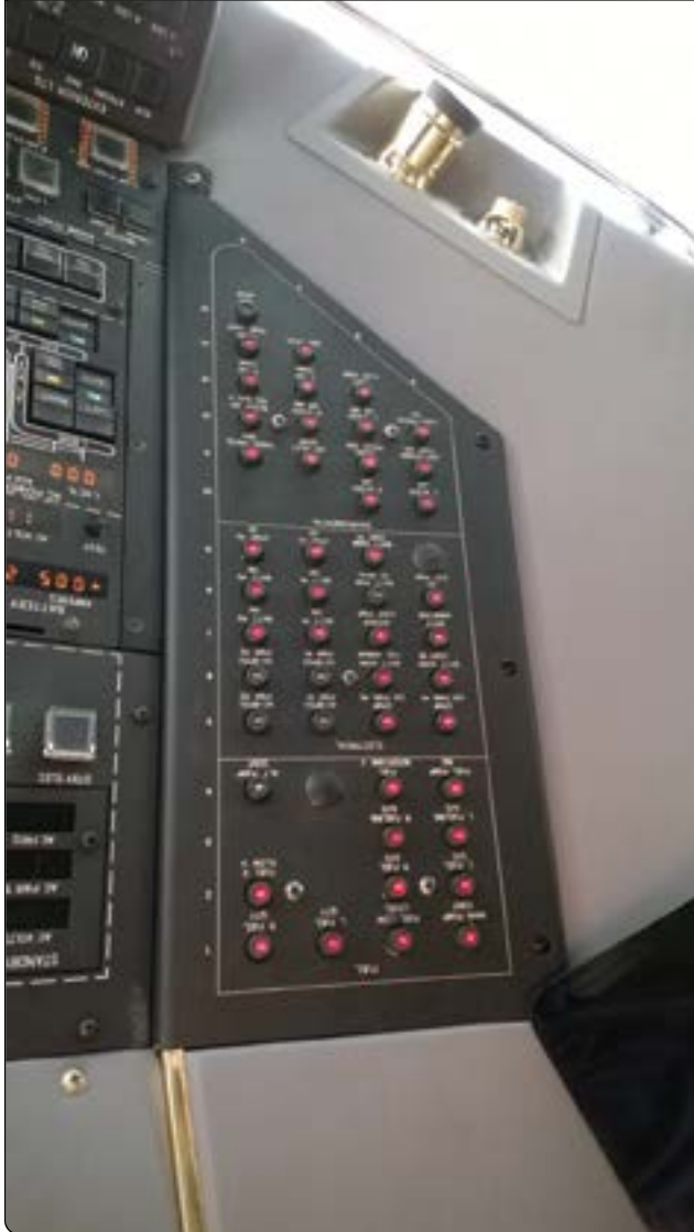
Figure 12-69. Circuit breaker assembly for aircraft electrical system.
