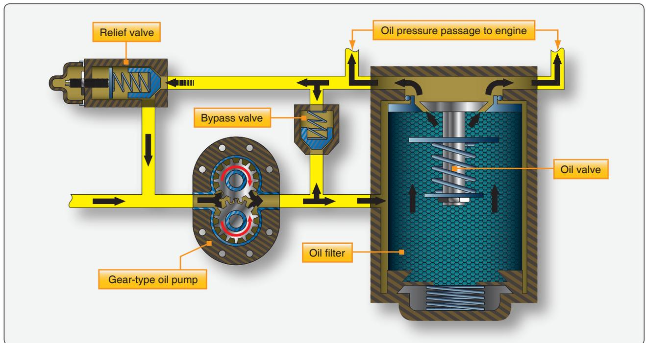
Figure 6-6. Engine oil pump and associated units.
