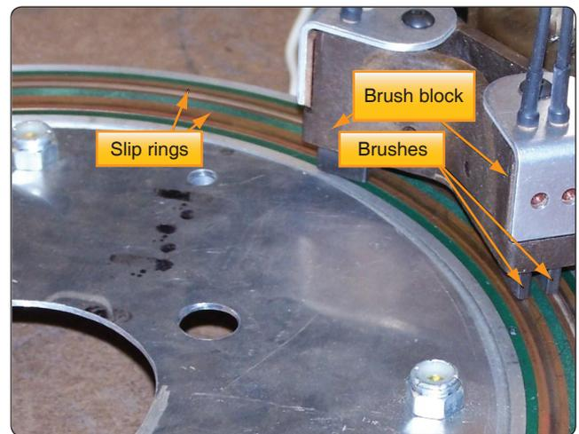
**Figure 7-29.** Deicing brush block and slip ring assembly.
