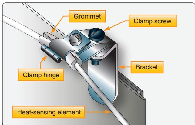
Figure 9-17. Inspection of fire detector loop clamp.
