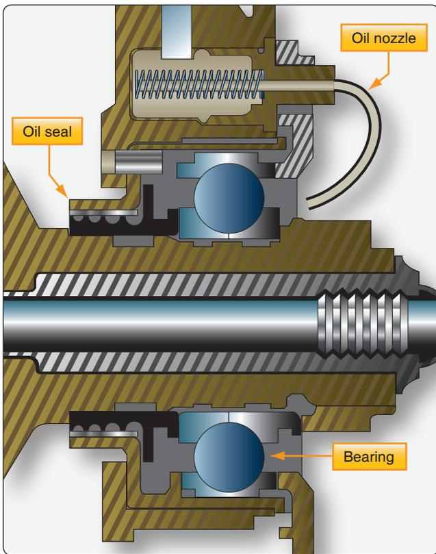
Figure 6-39. Oil nozzles spray lubricate on bearings.
