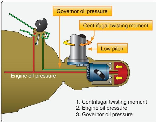
Figure 7-56. Diagram of hydromatic propeller operational forces.
