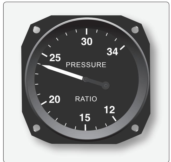
**Figure 10-72.** *Engine pressure ratio indications.*
