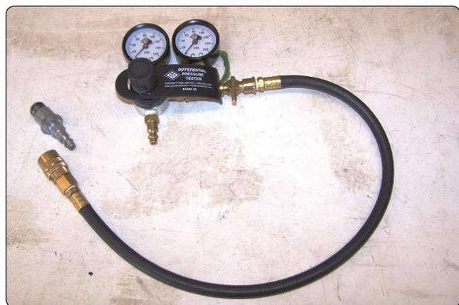
Figure 10-54. Compression tester and adapter.
