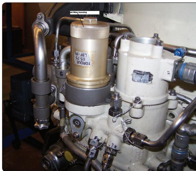
Figure 6-48. Oil filter housing.
