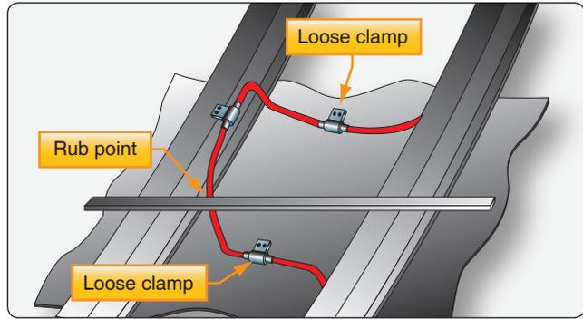
Figure 9-16. Rubbing interference.
