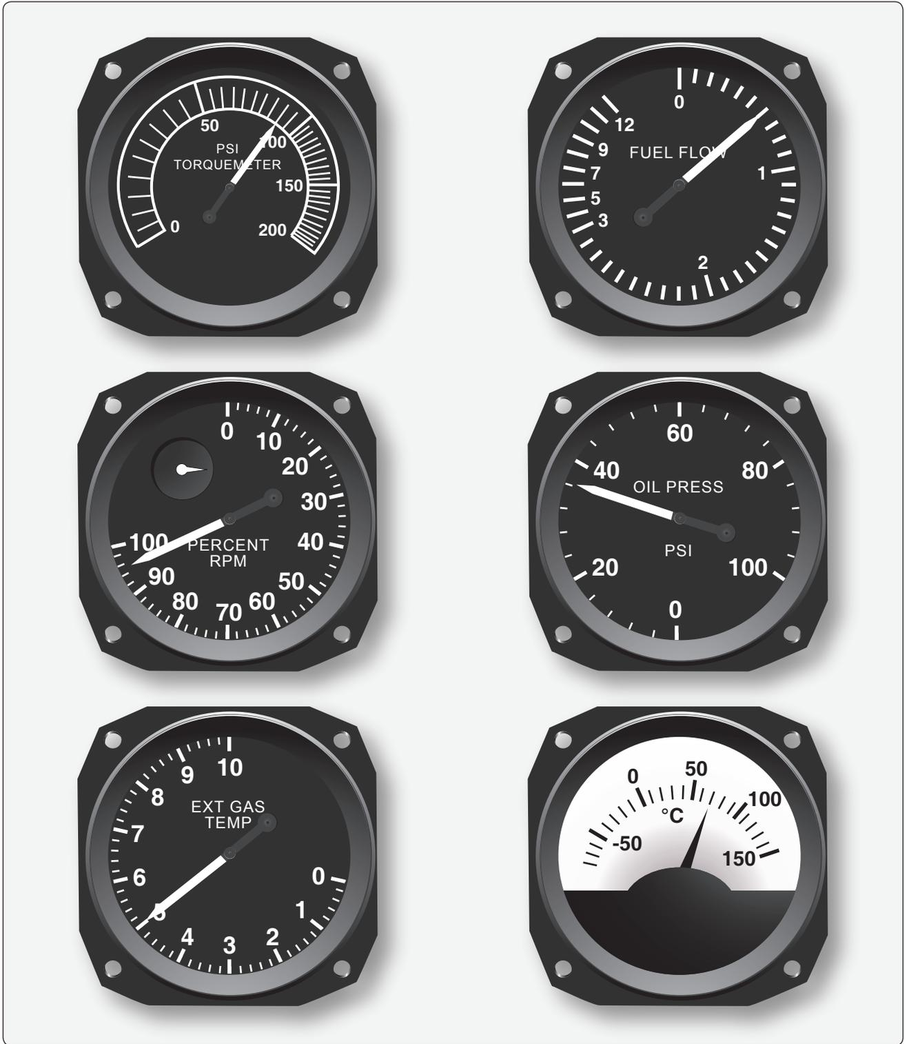
Figure 10-73. Typical turbine engine instruments.
