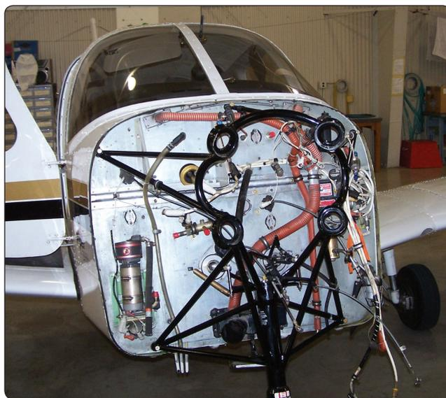
Figure 8-2. Typical firewall with components mounted on it.
