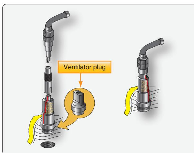
**Figure 8-20.** Ignition harness lead support installation.
