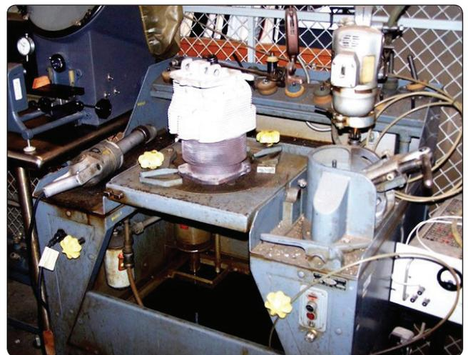
**Figure 10-16.** Valve seat grinding equipment.
