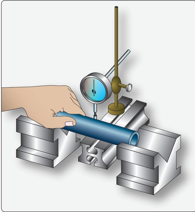
**Figure 10-14.** Checking a piston pin for bends.
