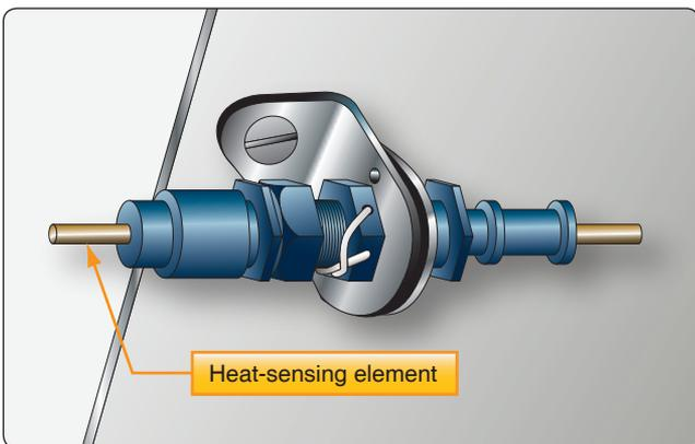
Figure 9-15. Connector joint fitting attached to the structure.
