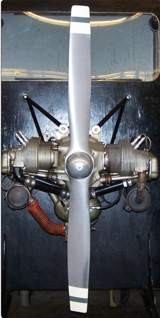
**Figure 7-11.** *Fixed-pitch propeller.*
