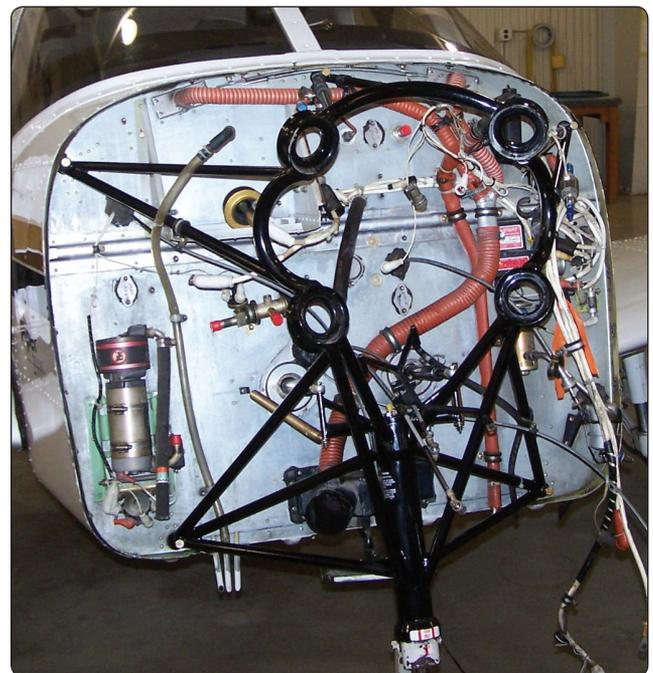
Figure 8-16. Engine mounting ring.
