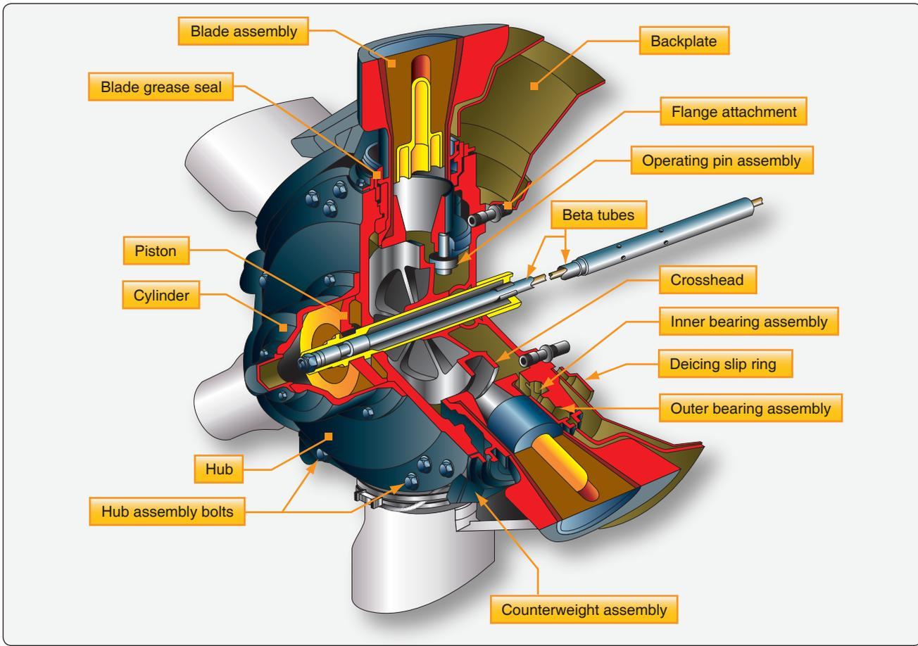
**Figure 7-47.** Turboprop propeller.
