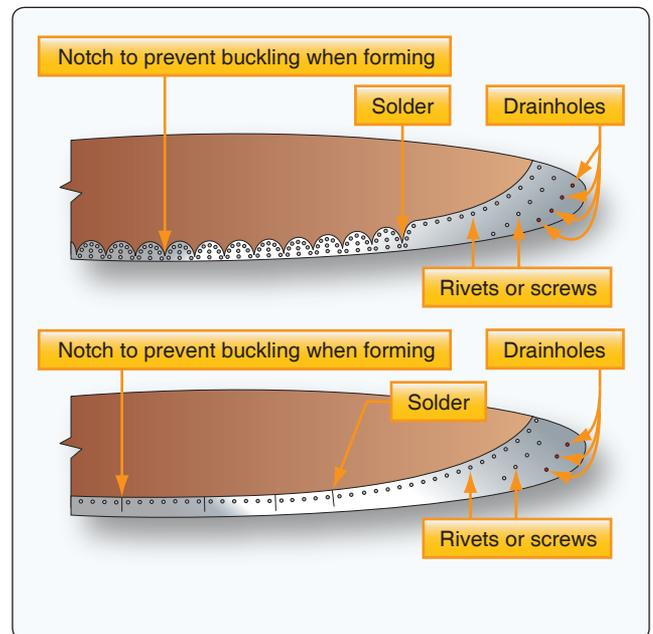
**Figure 7-21.** Installation of metal sheath and tipping.
