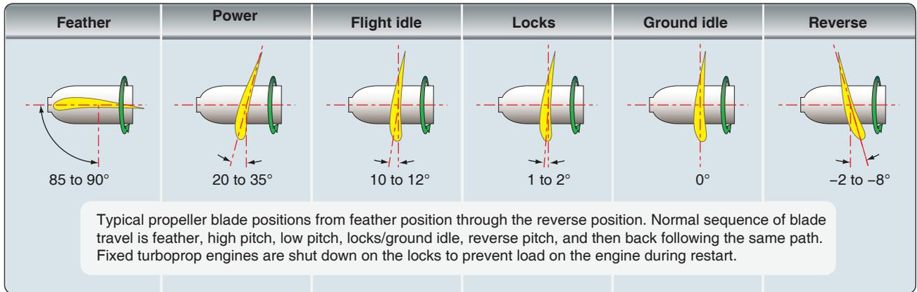
Figure 7-3. Propeller range positions.
