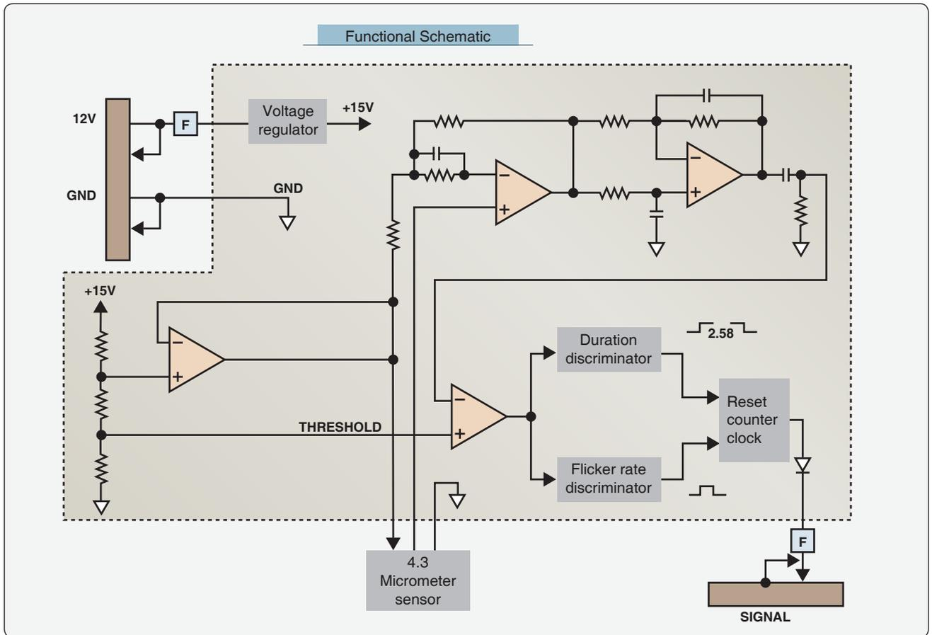
Figure 9-3. Optical fire detection system circuit.
