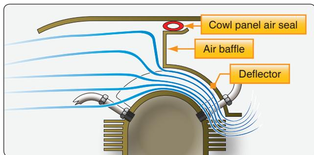
Figure 6-57. Cylinder head baffle and deflector system.
