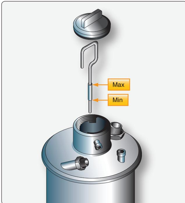
Figure 11-31. Oil dipstick minimum and maximum marks.
