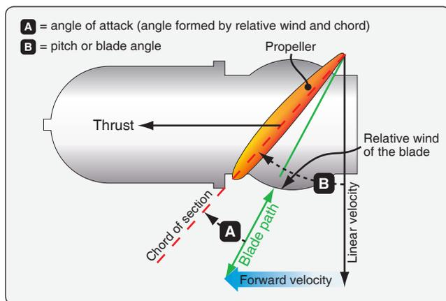
Figure 7-9. Propeller forces.
