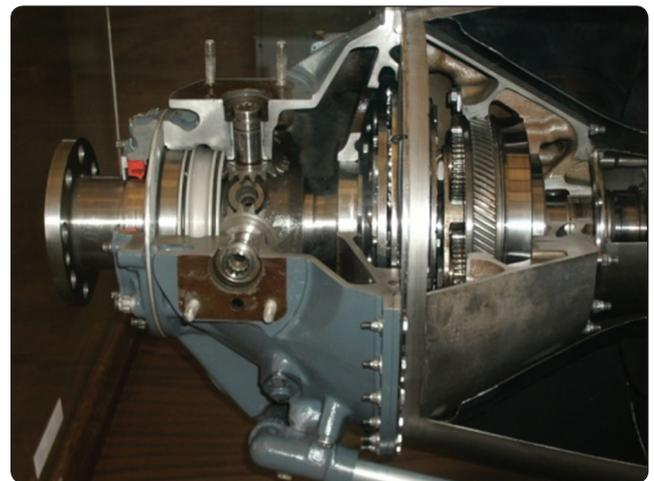
**Figure 7-46.** Reduction gearbox.
