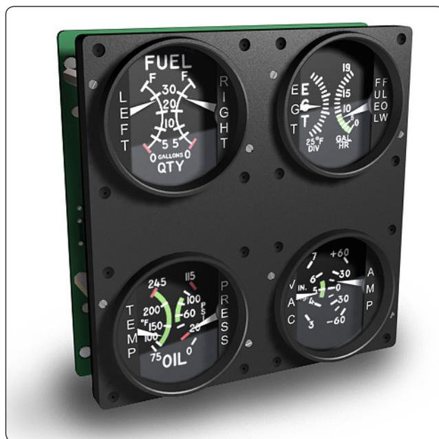
Figure 10-36. Engine instrument clusters.
