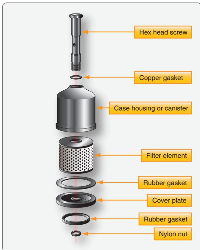
Figure 6-7. Housing filter element type oil filter.
