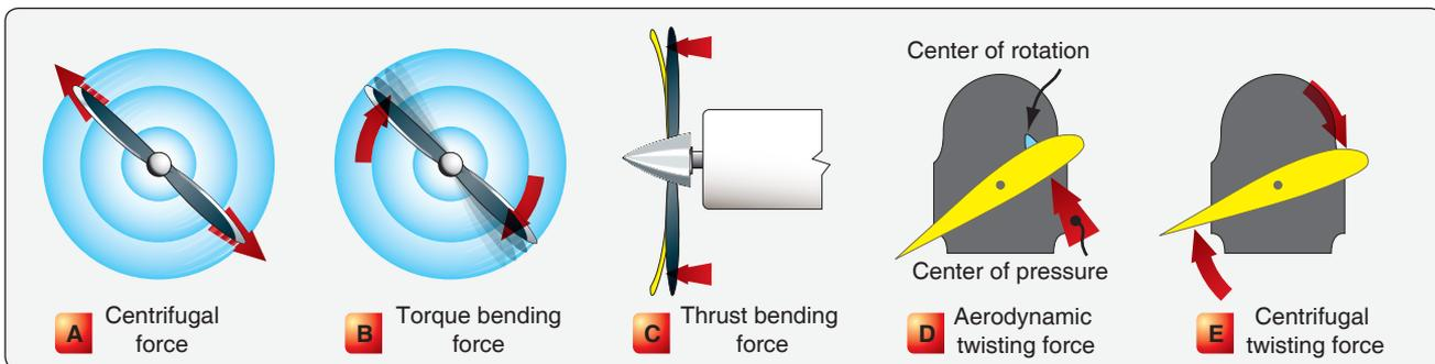
Figure 7-8. Forces acting on a rotating propeller.
