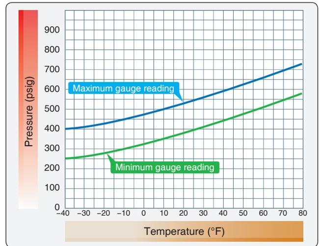
**Figure 9-18.** Fire extinguisher container pressure-temperature chart.
