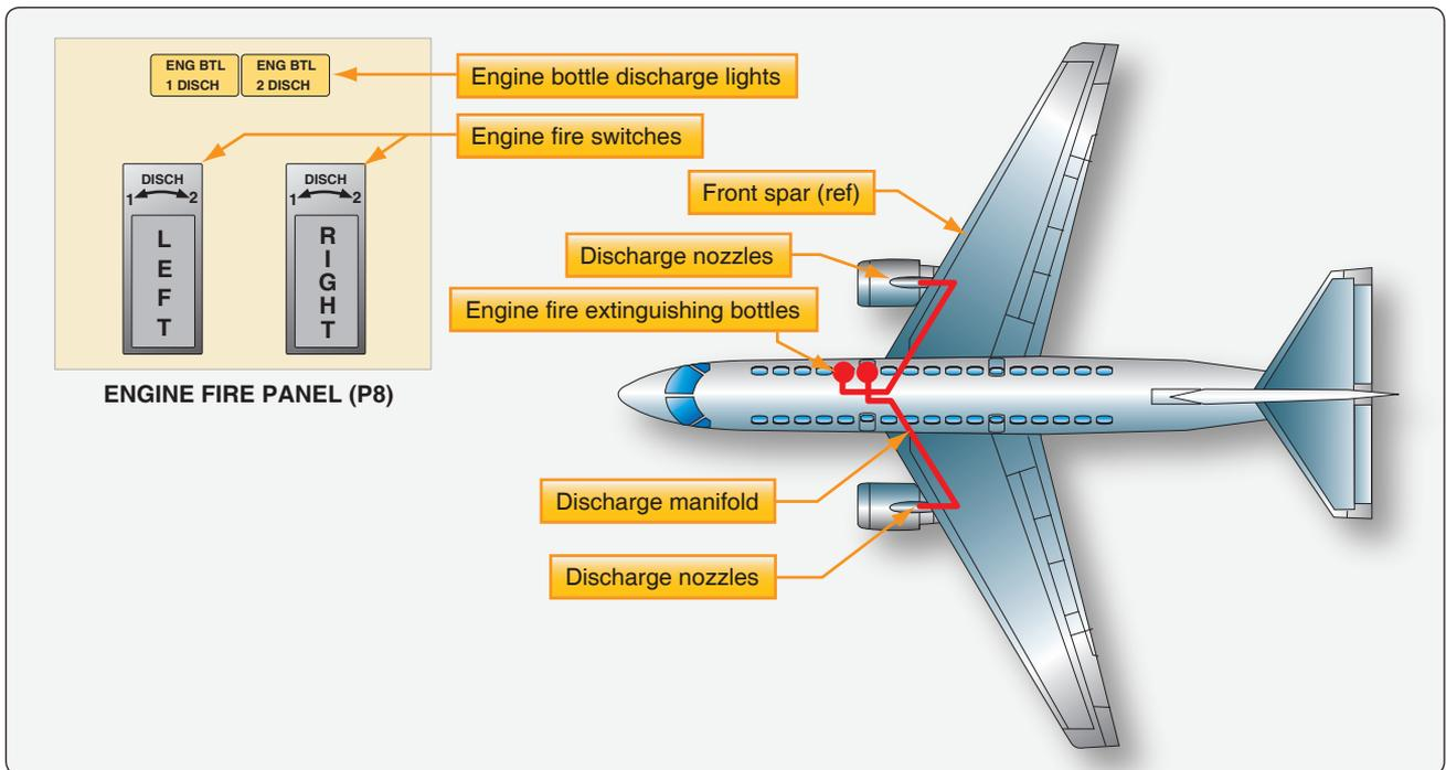
Figure 9-22. Boeing 777 fire extinguisher container location.
