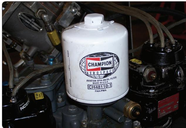
Figure 6-8. Full flow spin-on filter.
