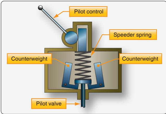
Figure 7-17. Underspeed condition.
