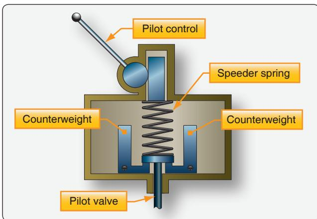
Figure 7-19. On-speed condition.
