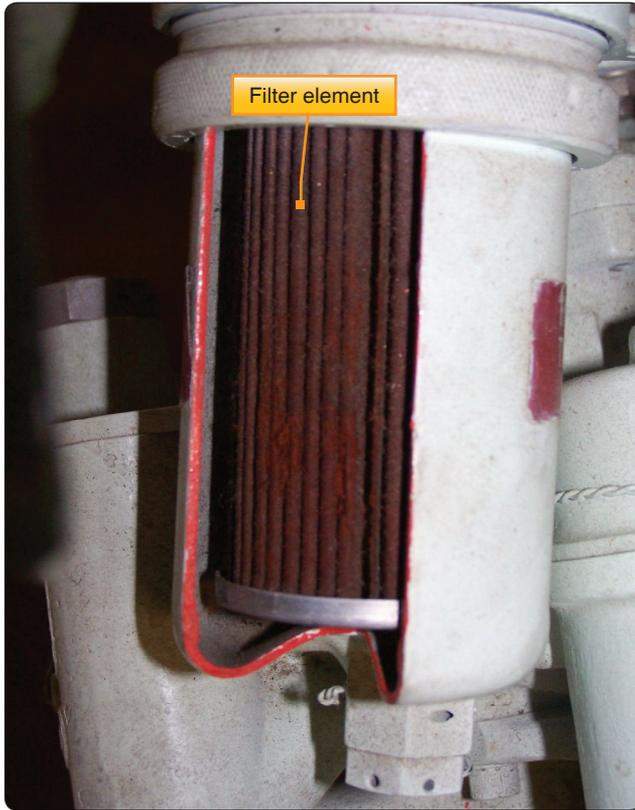
Figure 6-35. Turbine oil filter paper element.
