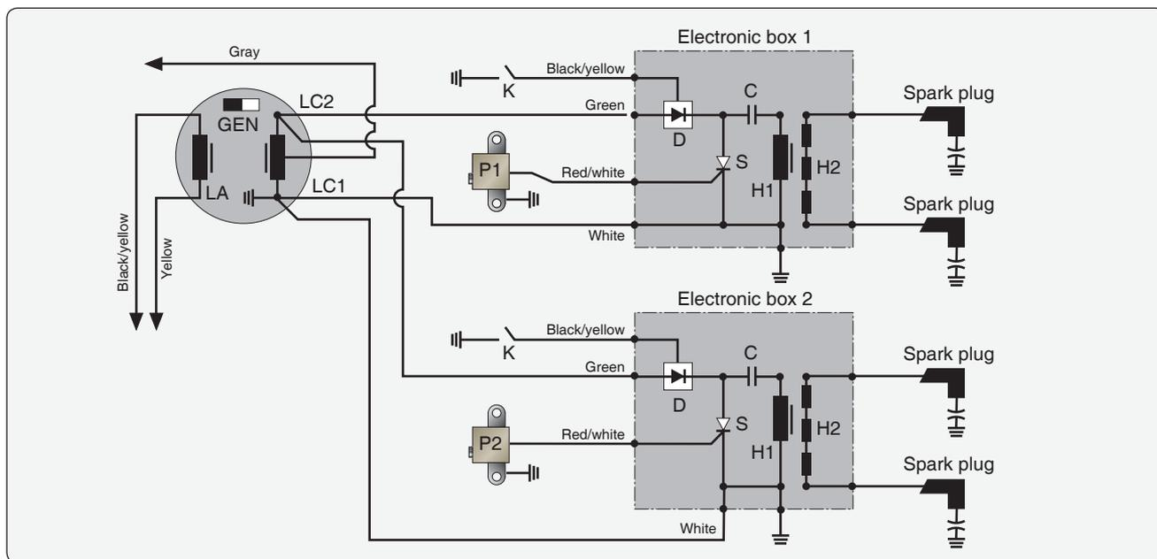
Figure 11-5 Rotax 503 and 582 electrical system.
