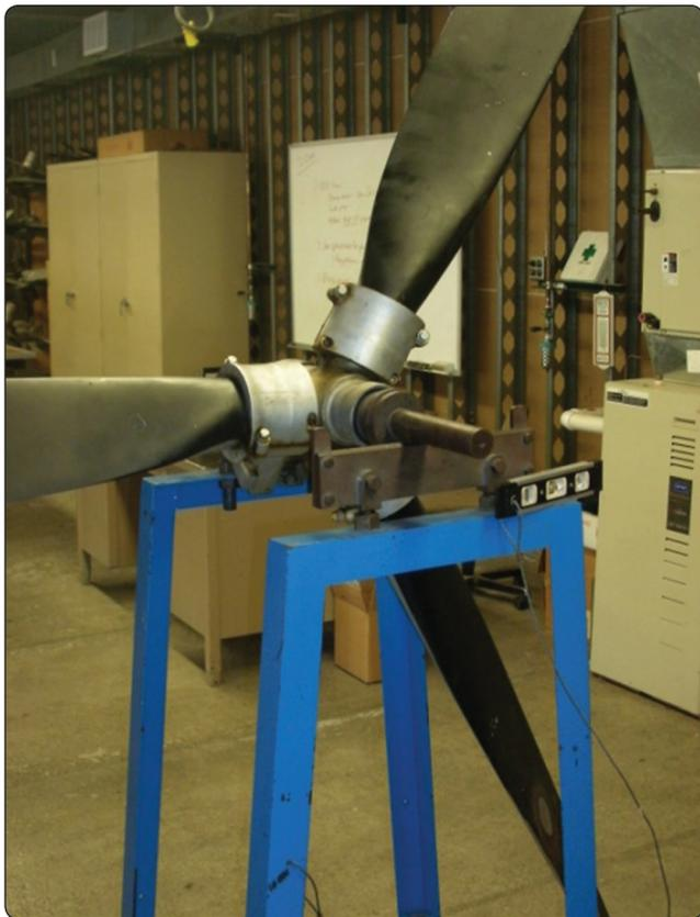
**Figure 7-40.** *Static propeller balancing.*
