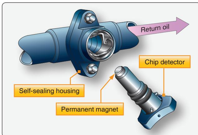
Figure 6-44. Chip detector.
