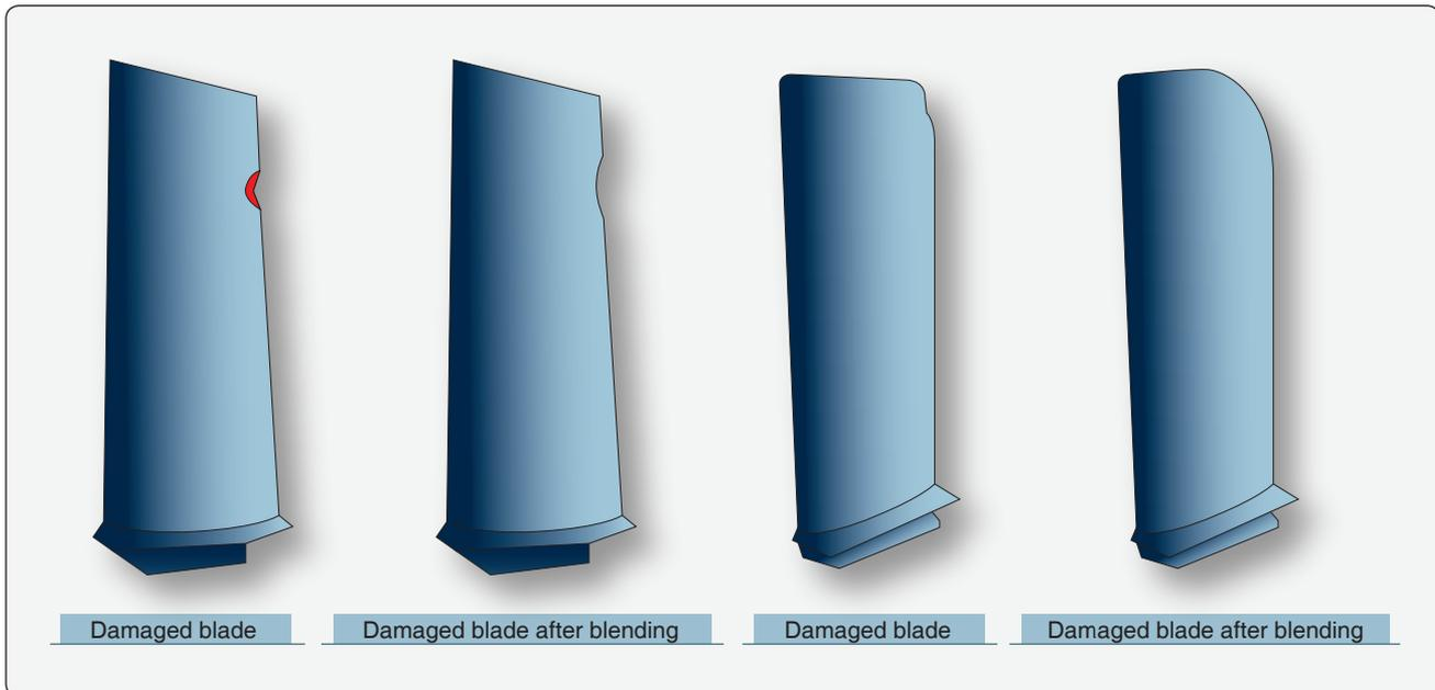
**Figure 10-58.** Examples of repairs to damaged blades.
