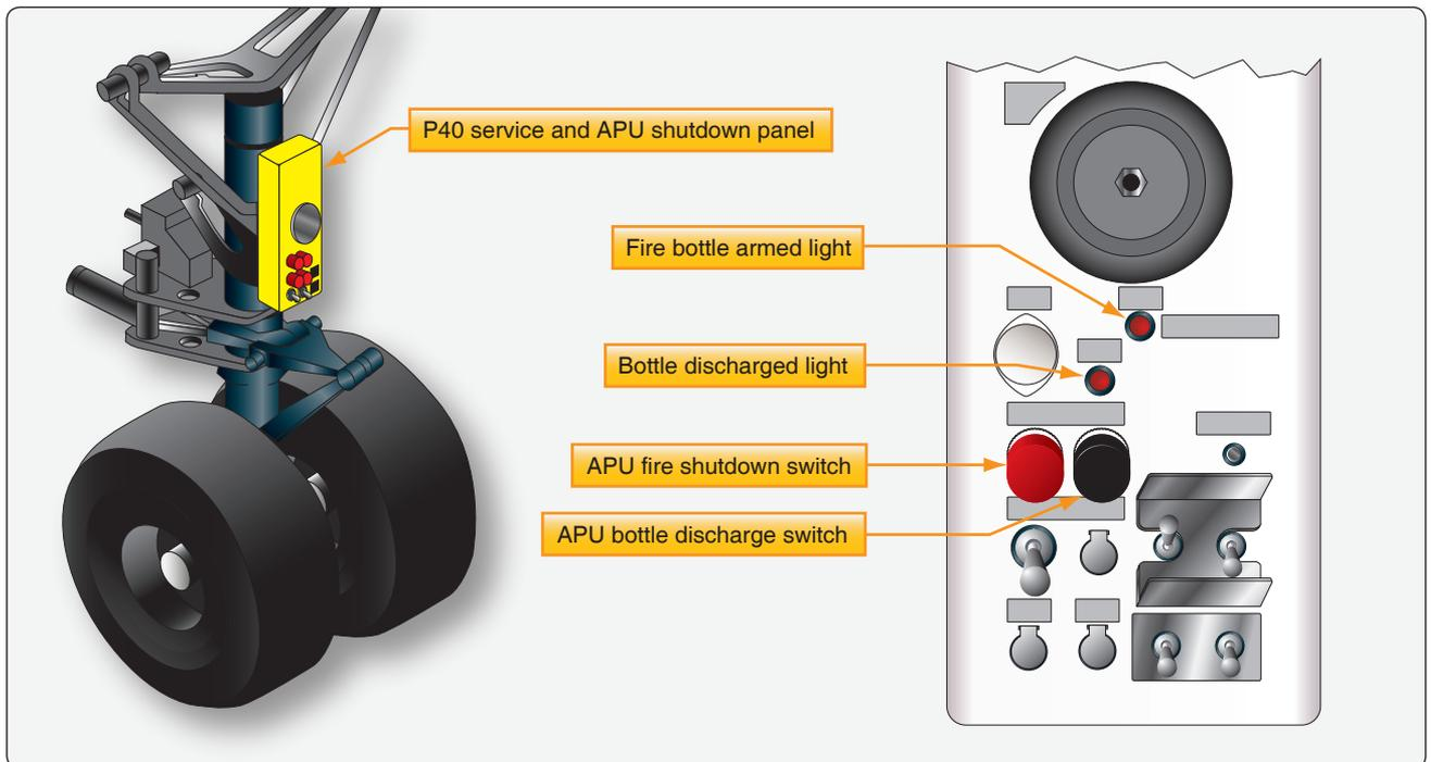
Figure 9-28. P40 service and APU shutdown panel.
