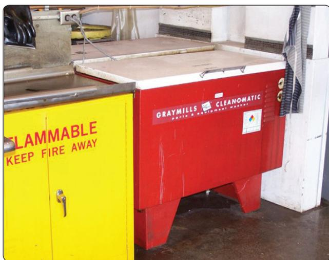
Figure 10-3. Typical solvent degreasing tank.
