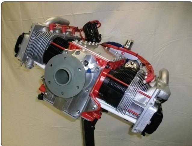
Figure 11-18. Aeromax direct drive, air-cooled, six-cylinder engine.
