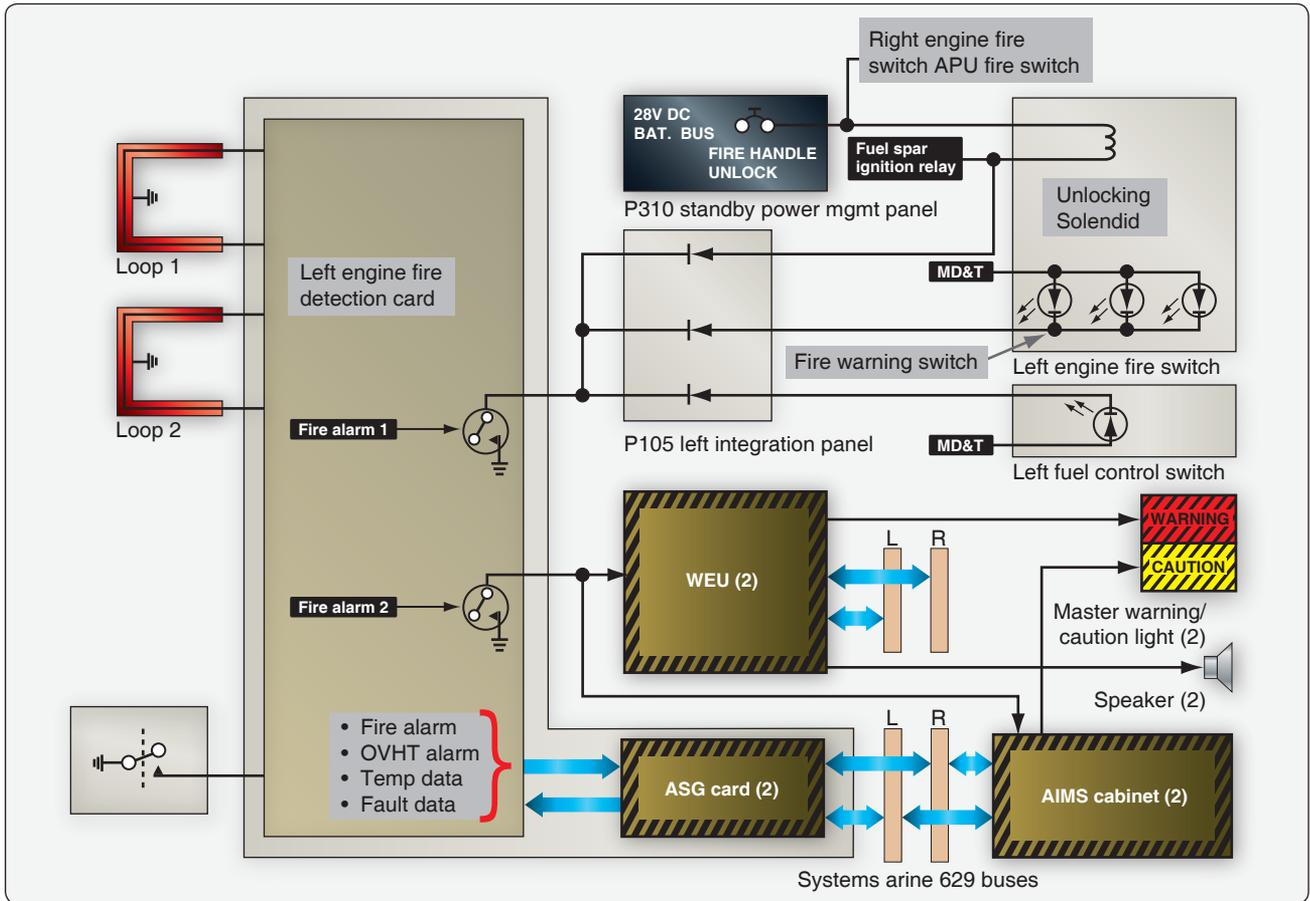
Figure 9-21. Engine fire detection system functional description.
