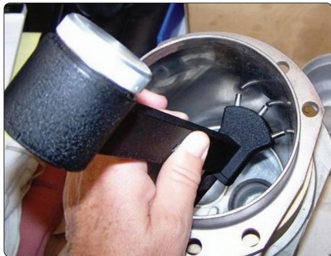
Figure 10-5. A cylinder bore gauge.
