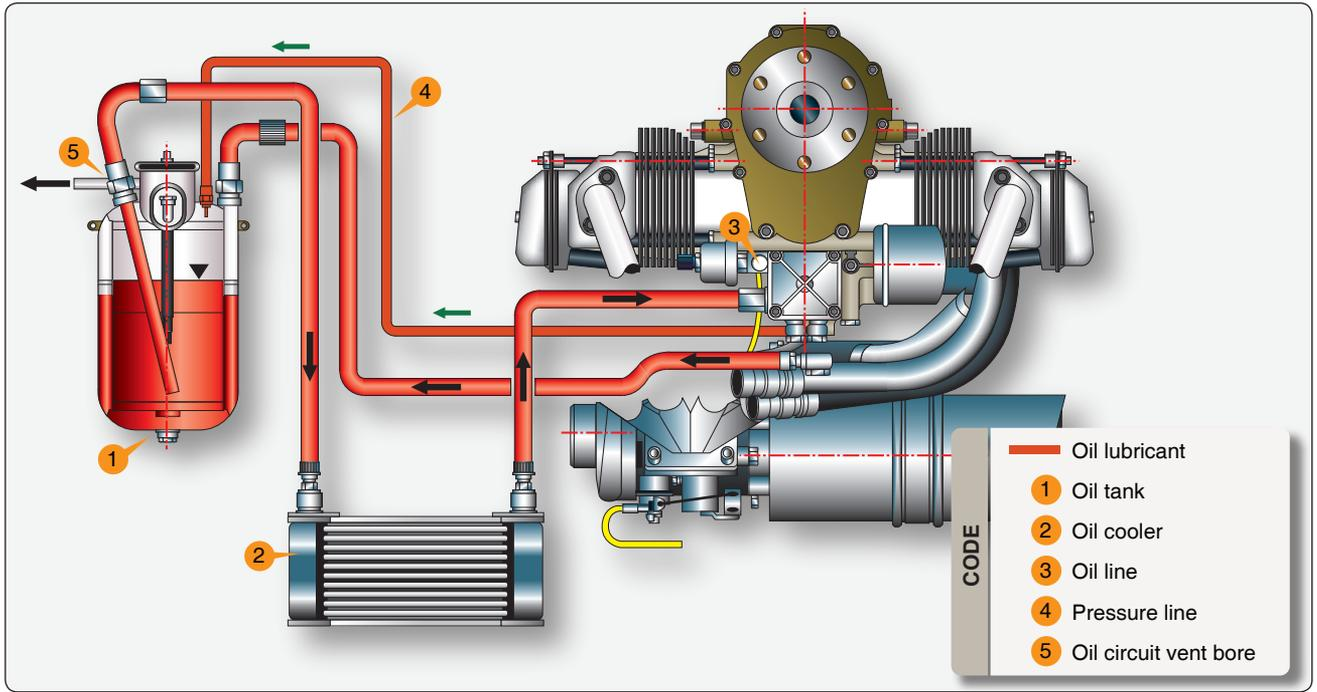
Figure 11-10. Lubrication system.
