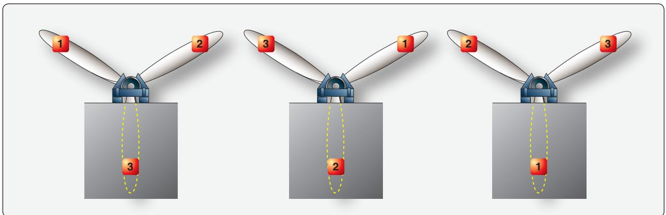
**Figure 7-39.** Positions of three-bladed propeller during balance check.
