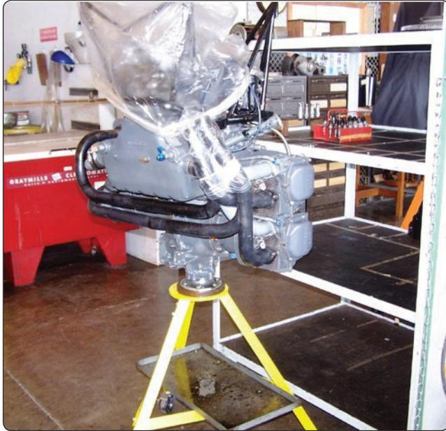
**Figure 10-1.** Engine mounted on an overhaul stand.
