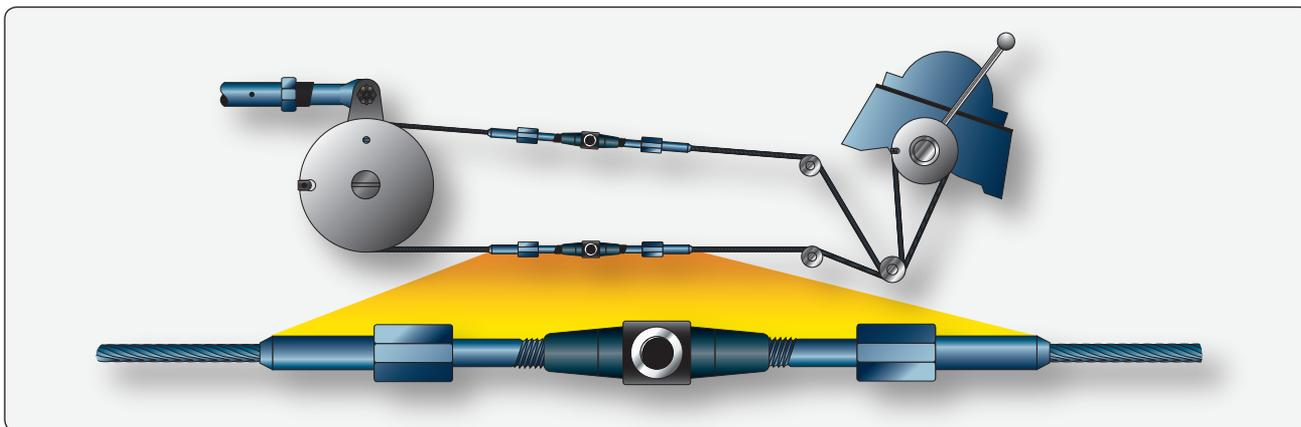
Figure 8-6. Engine control cable and turnbuckle assembly.
