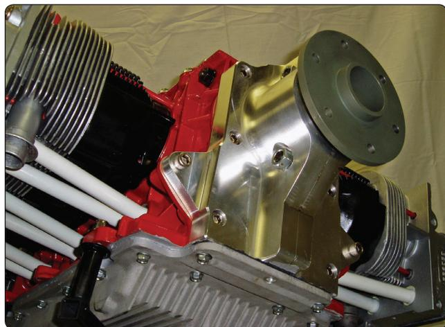
Figure 11-19. Front-end bearing on the 1000 IFB engine.
