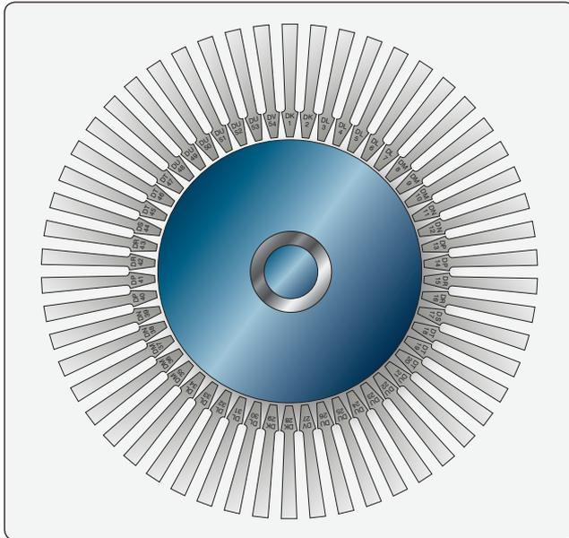
**Figure 10-67.** Typical turbine rotor blade moment-weight distribution.
