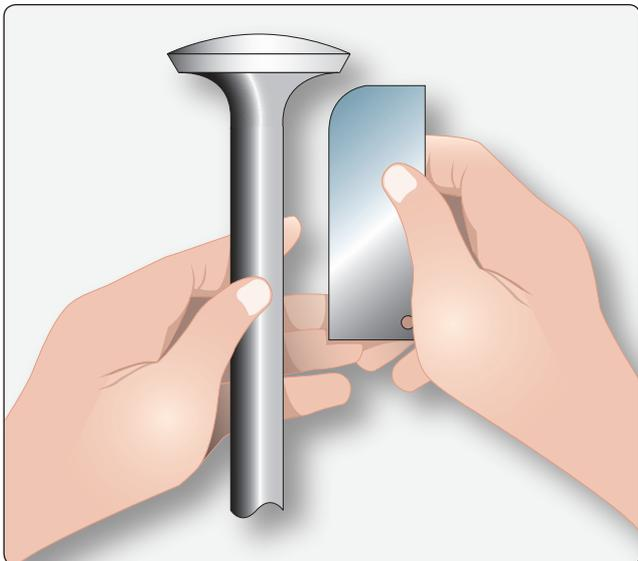
**Figure 10-8.** Checking valve stretch with a manufacturer's gauge.
