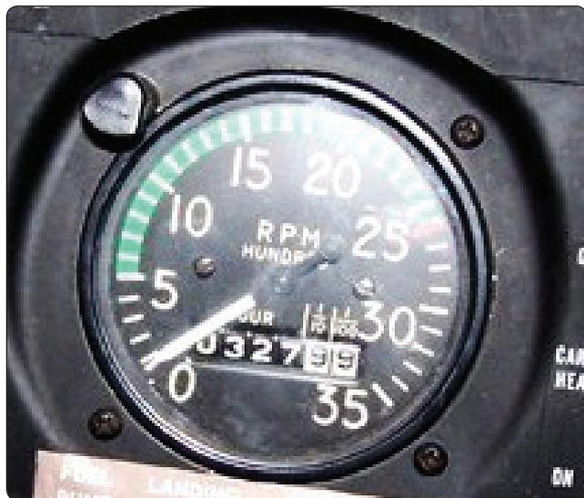
Figure 10-38. Tachometer.
