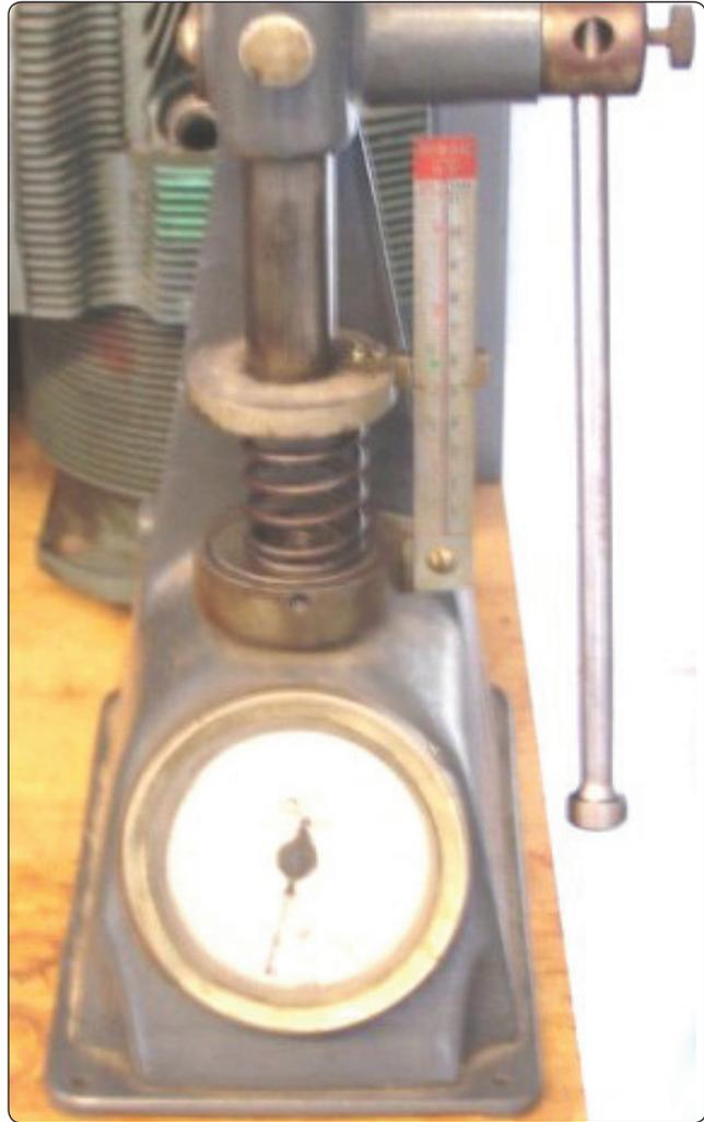
**Figure 10-9.** Valve spring compression tester.
