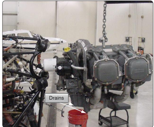
**Figure 8-4.** Oil system drain points.
