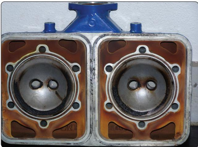
Figure 11-8. Water-cooled heads.
