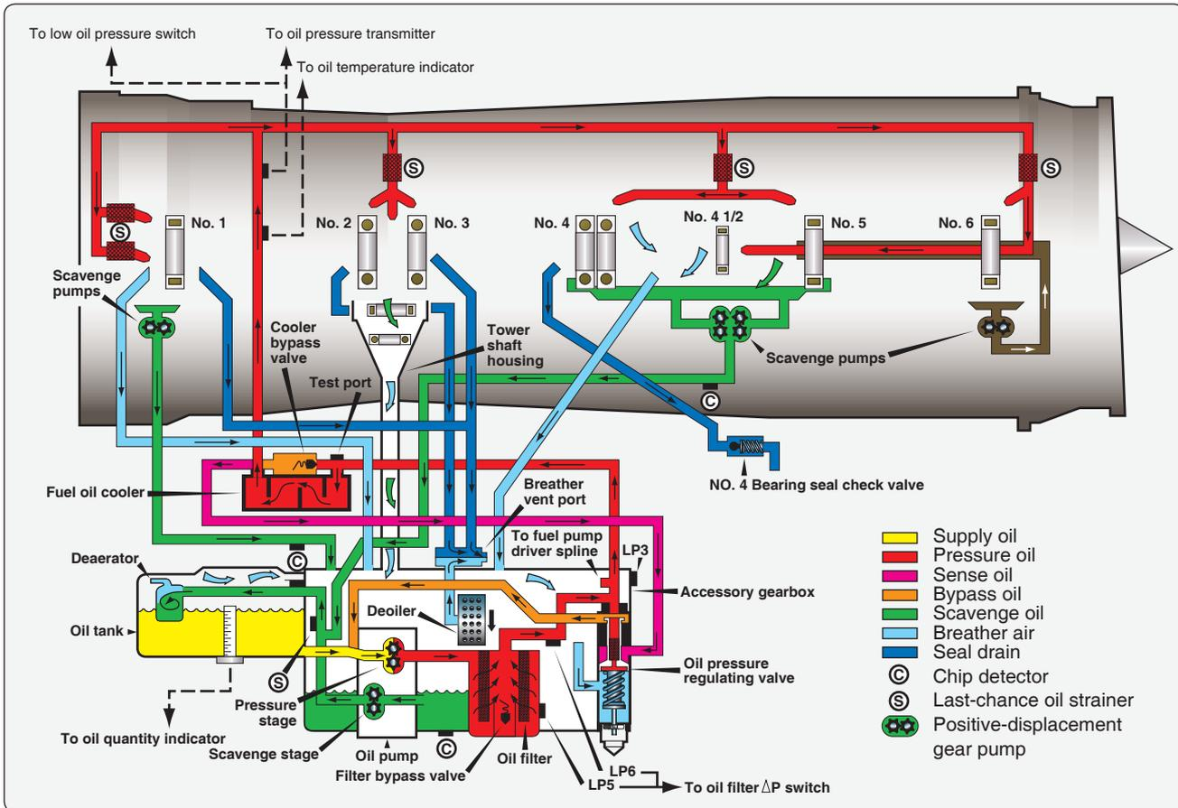
Figure 6-45. Typical turbine dry-sump pressure regulated lubrication system.
