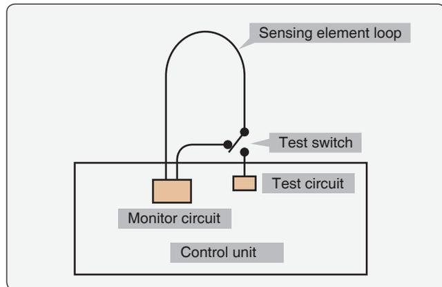
Figure 9-6. Continuous-loop fire detection system test circuit.
