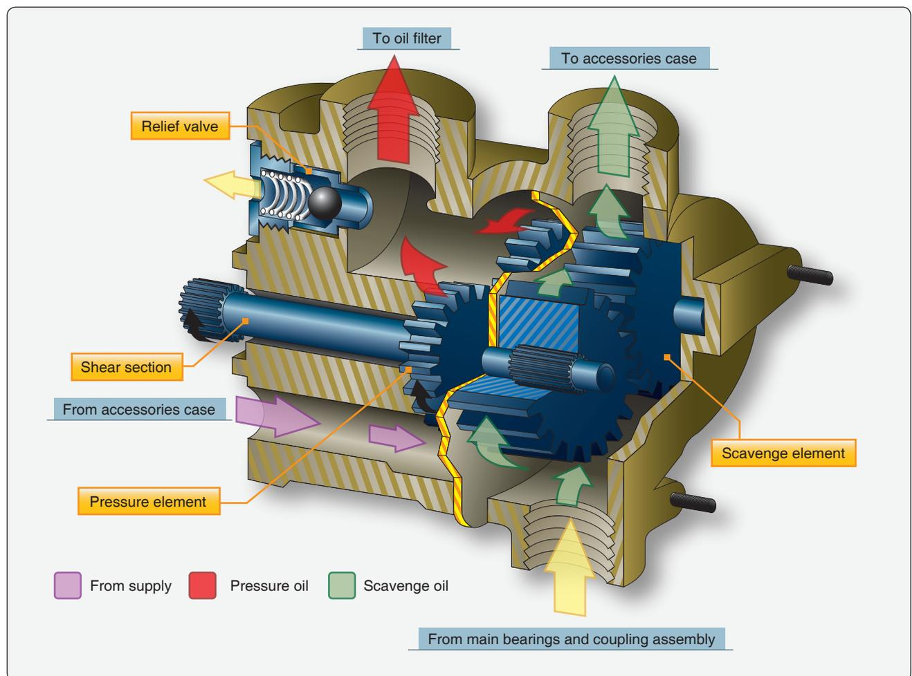
Figure 6-32. Cutaway view of gear oil pump.
