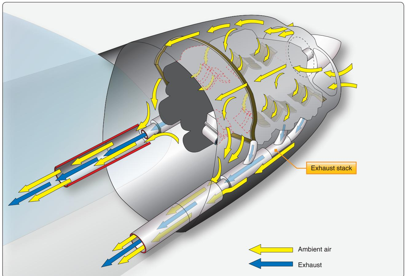
Figure 6-53. Engine cooling and exhaust system.
