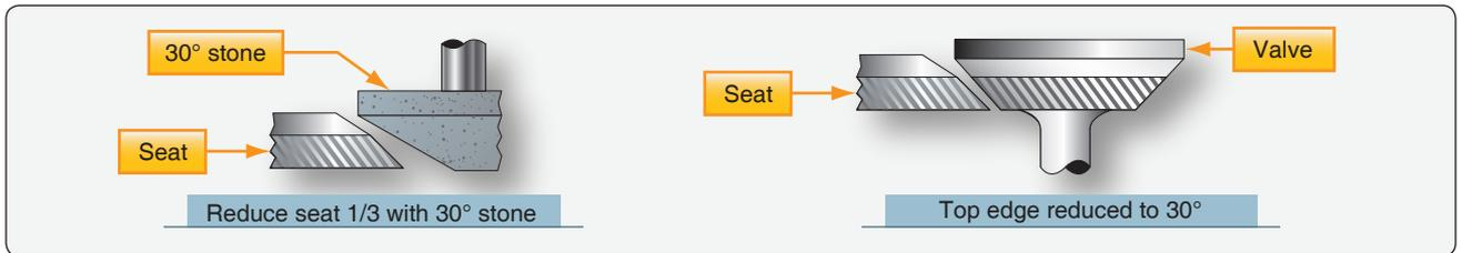
**Figure 10-20.** Grinding top surface of the valve seat.
