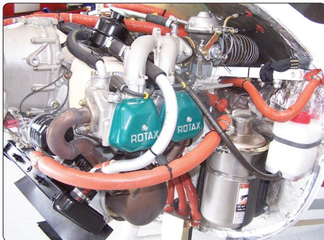
**Figure 11-6.** Typical four cylinder, four-stroke horizontally opposed engine.
