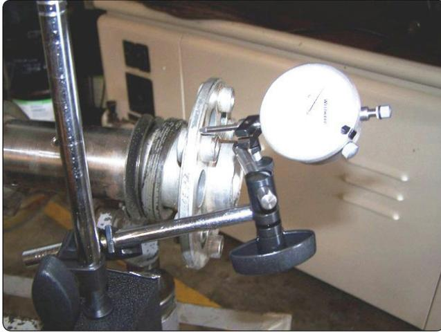
Figure 10-10. Checking crankshaft runout.
