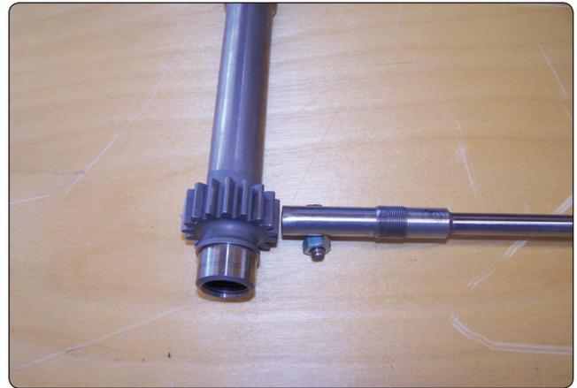
Figure 10-79. Magnetic pickup and gear.
