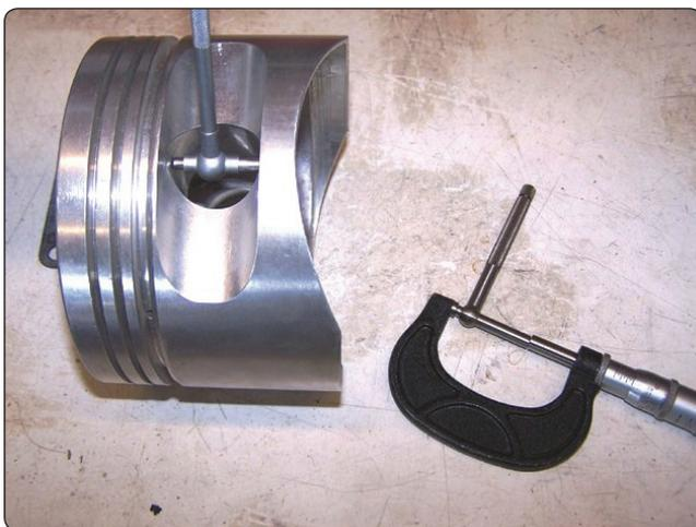
Figure 10-12. Telescoping gauges and micrometer combination.
