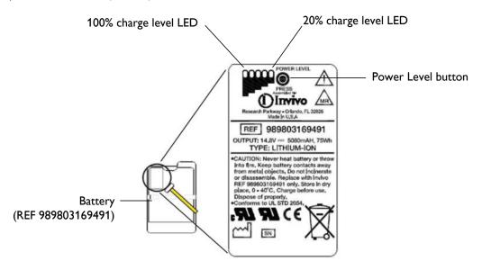
The module batteries must be charged by Invivo battery charger (REF 989803152891). Refer to the instructions and cautions provided with the charger for information. The minimum voltage for module battery is 3.4 Vdc.
