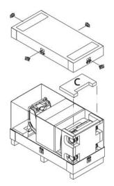
2. Remove the accessories box and foam insert B.
