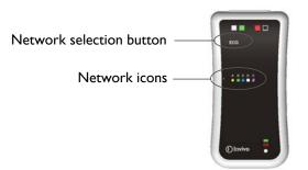
To make it as easy as possible to press and release the button while observing the network icons, either place the module on a flat steady surface, or hold the module as shown in the figure right, and use your thumb to press the network selection button.
