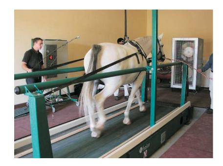
The rear of the treadmill has designed so that dung is guided handled away from the belt. This makes it easier for daily cleaning inside and out.
