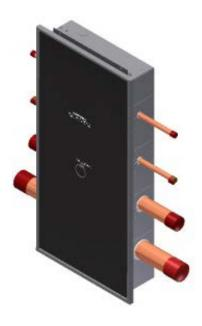
Shown above VU42A2N3O4V 4 valve box with gauges 1/2" Medical Air, 1/2" N2O, 3/4" Oxygen, 1" Medical Vacuum
