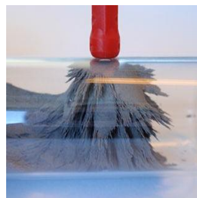
Figure 3. Attraction of ferrofluids by magnets.
