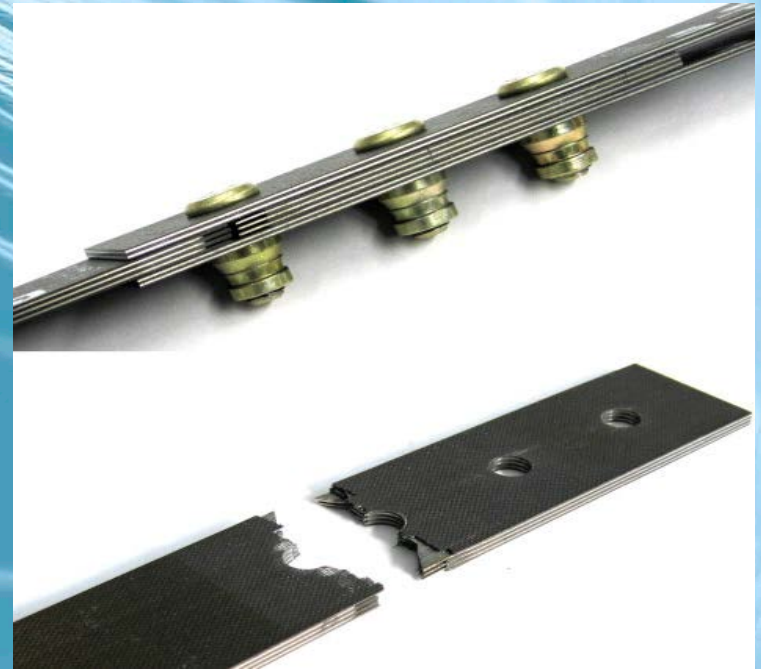
CFRP/titanium hybrid material for improving composite bolted joints. B. Kolesnikov et al.
