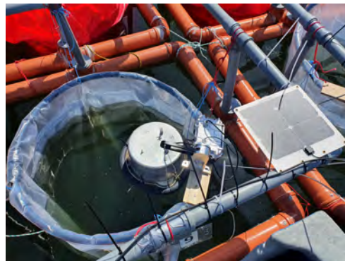
Lifting device for swimming chamber with attached sensors and control device connected to a solar panel. ©Eti Levi
