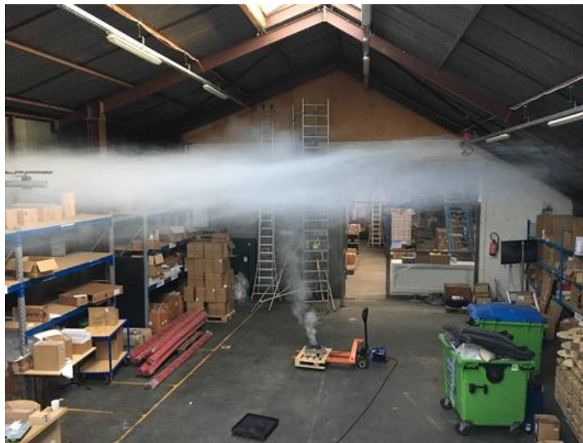
Figure 8: Image of stratification of a TF2 test during a summer day in a warehouse facility
