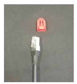
• For UTP/STP cable with the RJ45 connector already attached mount the connector guard. The connector guard is there to protect the cable gasket from tearing.
