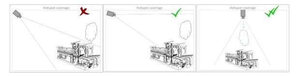
**Redundancy**: Make sure the FOV's of the cameras have enough overlap.
