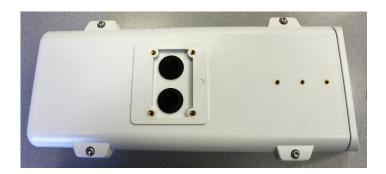
• Push the UTP/STP cable and ALARM cable down so that the cable gasket adjust itself on the cable. Make sure the gaskets are fitted properly.
