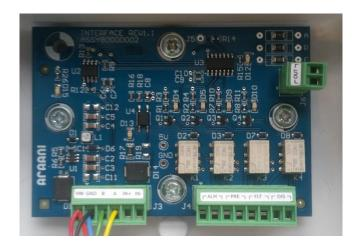
The IO connections are located on the dedicated Araani Interface board and are provided for interconnection with third party equipment.
