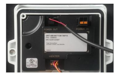
The solution should be powered using the POWER-IN terminal with a dedicated power supply. The POWER-IN terminal is rated for 12-28VDC operation and is polarity free.
