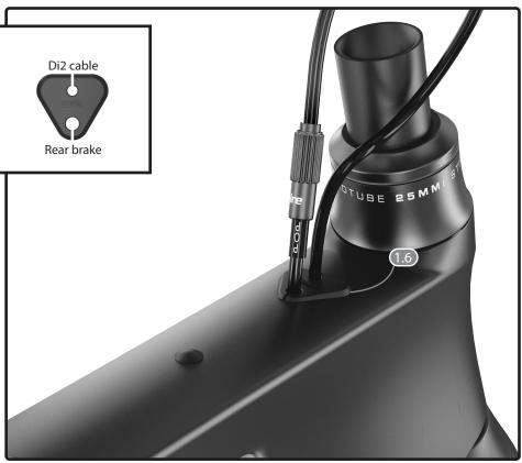
Use the proper grommet on the top tube to fix the cable correctly, depending if you use mechanical drive-train (1.5) or electronic shifting (1.6).
