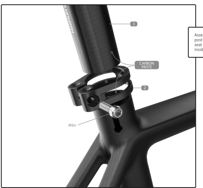
Assemble the seat post collar (2) with the seat post (3). Apply carbon paste inside the frame's seat tube and on the seat post where it inserts inside the frame. Tighten the bolt at 4 Nm.
