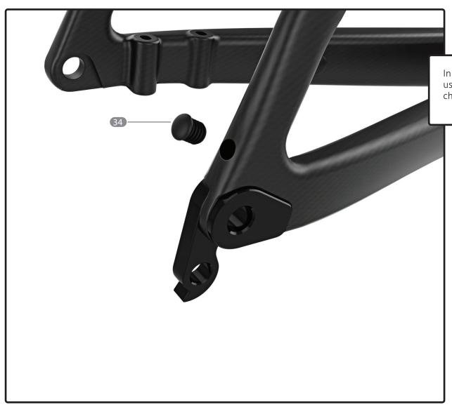
In the wireless groupset configuration, use the Round Plug (34) to plug the chain stay hole.
