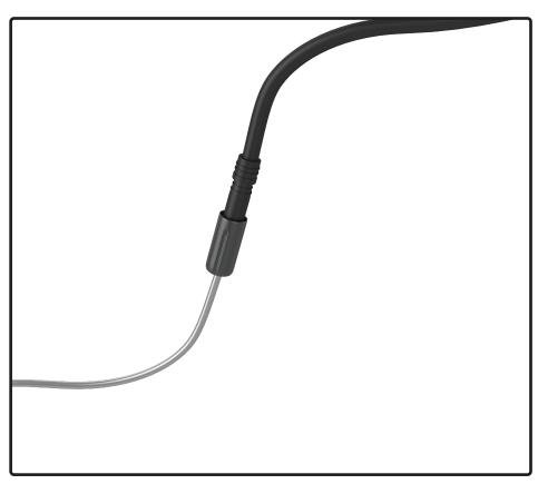
The Di2 cable routing can be achieved easily using this simple trick: use a gear cable and a metal cable end to fix the Di2 cable. For more information on Shimano Di2 electronic system installation, go to: si.shimano.com.
