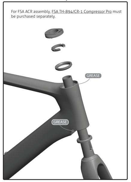
IMPORTANT: No more than 30mm of spacers can be placed between the stem and the top cap. The steerer must be trimmed no more than 5mm above the stem. The use of more than 5mm of spacers above the stem could void the efficiency of the compressor and void the warranty.
