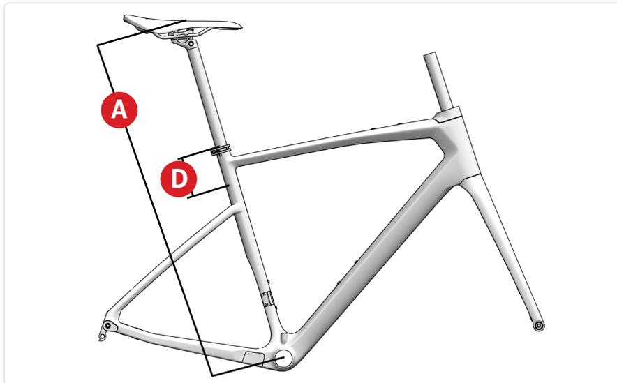
Refer to the adjacent table for details on saddle height and seatpost insertion limits:
