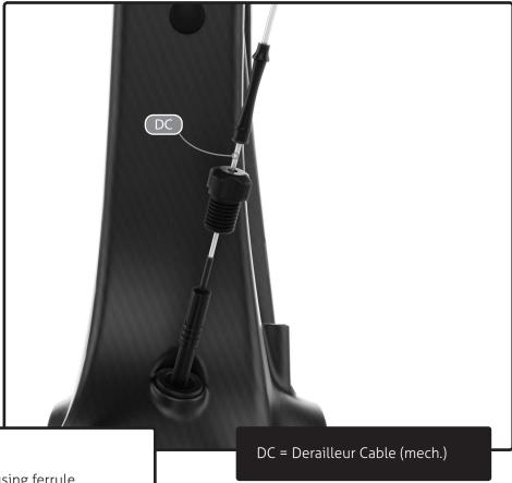
Enter derailleur housing through bottom bracket (BB) hole.
