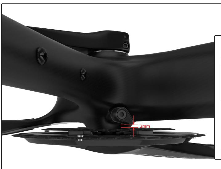
1. Select the corresponding chain catcher. The selection of the correct chain catcher is made according to the size of the small chaining.
