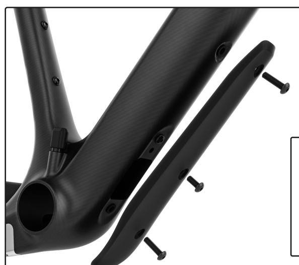
The cable stop need to be in place to fix the downtube protector.
