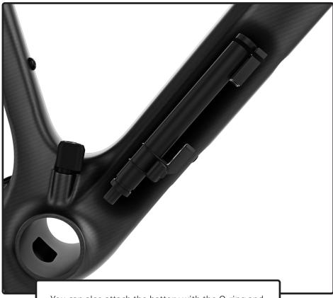
You can also attach the battery with the O-ring and the junction box with a tie-wrap on the groove of the battery and insert the package through the hole. This allow you to use a dropper post.
