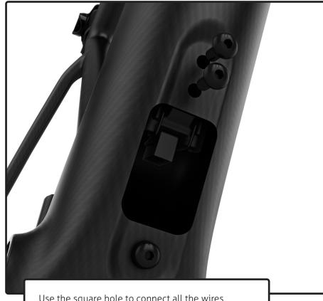
Use the square hole to connect all the wires to the junction box.
