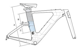
Refer to the tables below for details on Saddle Height and SeatPost insertion limits.
