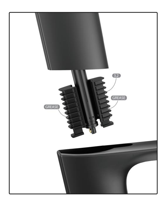
The Di2 battery is hidden in the seatpost; use the Di2 battery holder (3.2) to fix the battery correctly. Apply a slight amount of grease on both parts.
