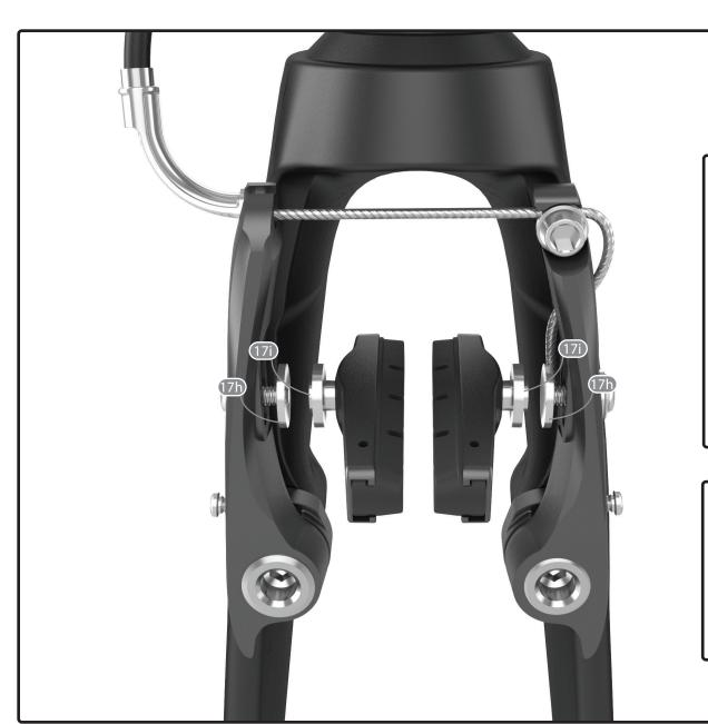
IMPORTANT: Depending on brake pad spacing or rim width, the brake arm may rub on the frame down tube. Make sure the pad spacing is appropriately adjusted.
