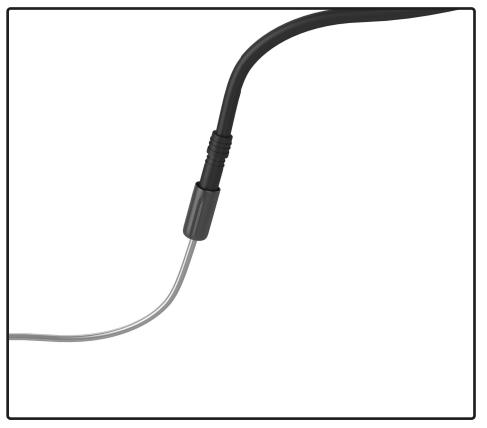
The Di2 cable routing can be achieved easily using this simple trick: use a gear cable and a metal cable end to fix the Di2 cable. For more information on Shimano Di2 electronic system installation, go to: si.shimano.com.
