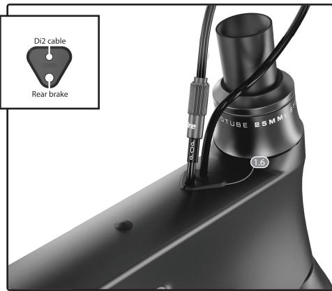
Use the proper grommet on the top tube to fix the cable correctly, depending if you use mechanical drive-train (1.5) or electronic shifting (1.6).
