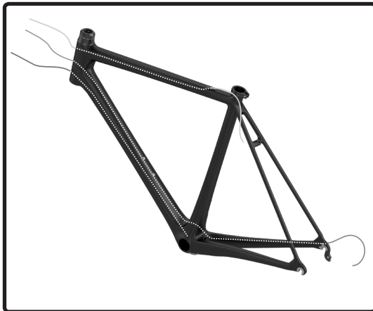
4. Cable housing installation
