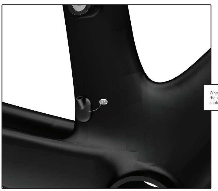
When using an electronic drive-train, use the grommet (13) to fix the front derailleur cable.
