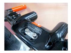
q. Untighten fairing clamp bolts, remove the parts just installed and cut steer tube to proper length.
