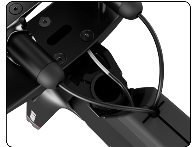
3. Ensure mechanical drivetrain cables are routed through the TTB's top and into the frame.
