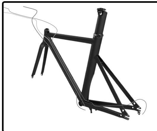
2. Cable housing installation
