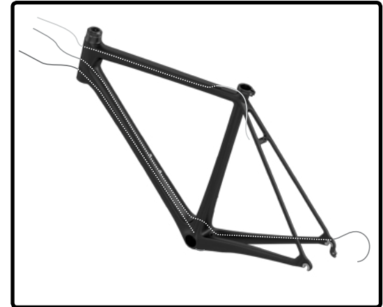
3. Cable housing installation
