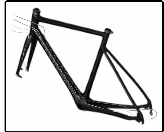
3. Cable housing installation
