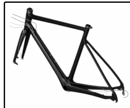
3. Cable housing installation
