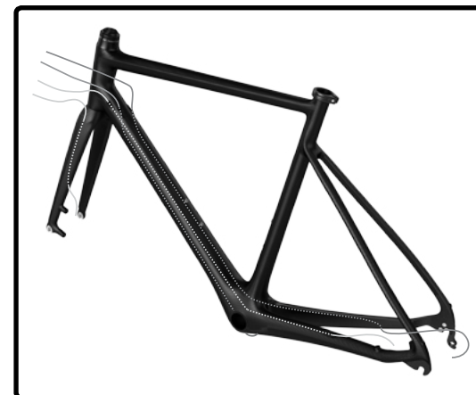
3. Cable housing installation
