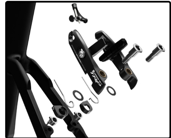
6. Rear brake installation
