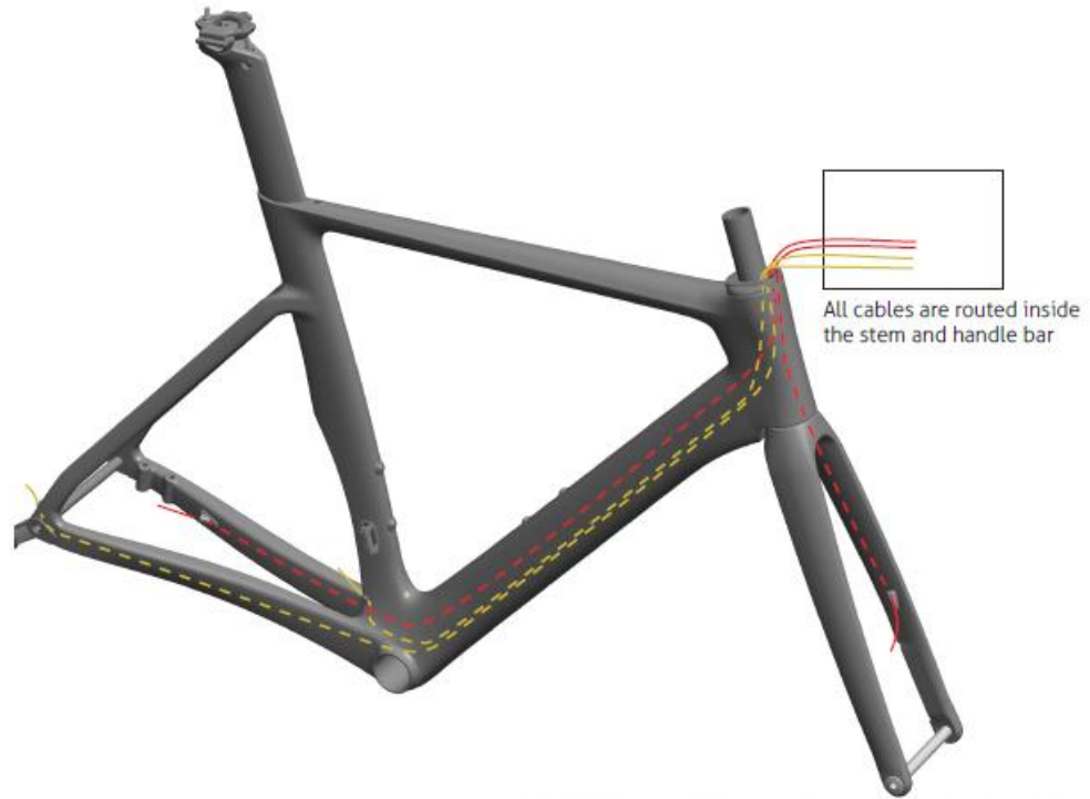
Red line: brake cable/housing / Yellow line: derailleur cable/housing Cable routing with option 1.
