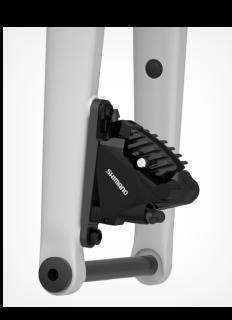
Flat mount disc brakes Standard version on both frames, for 140 and 160 mm rotors.
