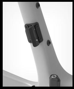
$\label{lem:continuous} Riveted\ Front\ Derailleur\ Hanger \\ \textit{Stiff}\ and\ light.$
