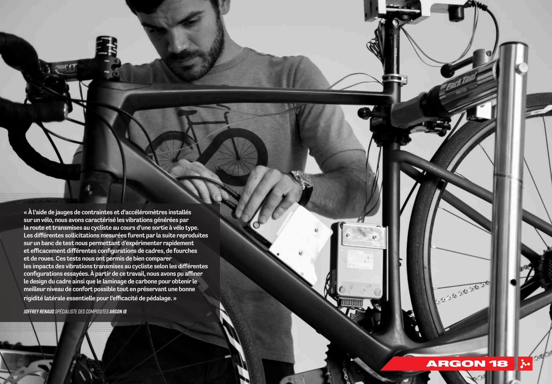
A black and white photograph of a man with a beard, wearing a t-shirt with a bicycle graphic, working on a bicycle frame. The frame is mounted on a stand. Several sensors and wires are attached to the frame, particularly around the bottom bracket and rear triangle. The man is looking down at the sensors. The background is a plain, light-colored wall.
