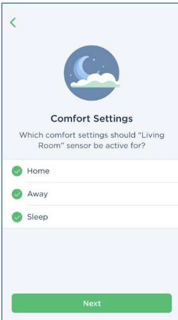
**What are Comfort Settings?** When a sensor participates in a Comfort Setting its temperature readings are used in tandem with the thermostat's readings to calculate an average temperature across multiple rooms.
