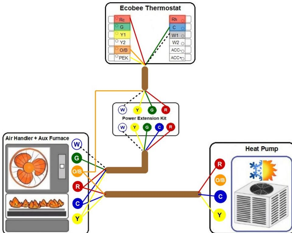
Diagram 17. Heatpump (2-stage) + Aux Heat (1-stage) using PEK
