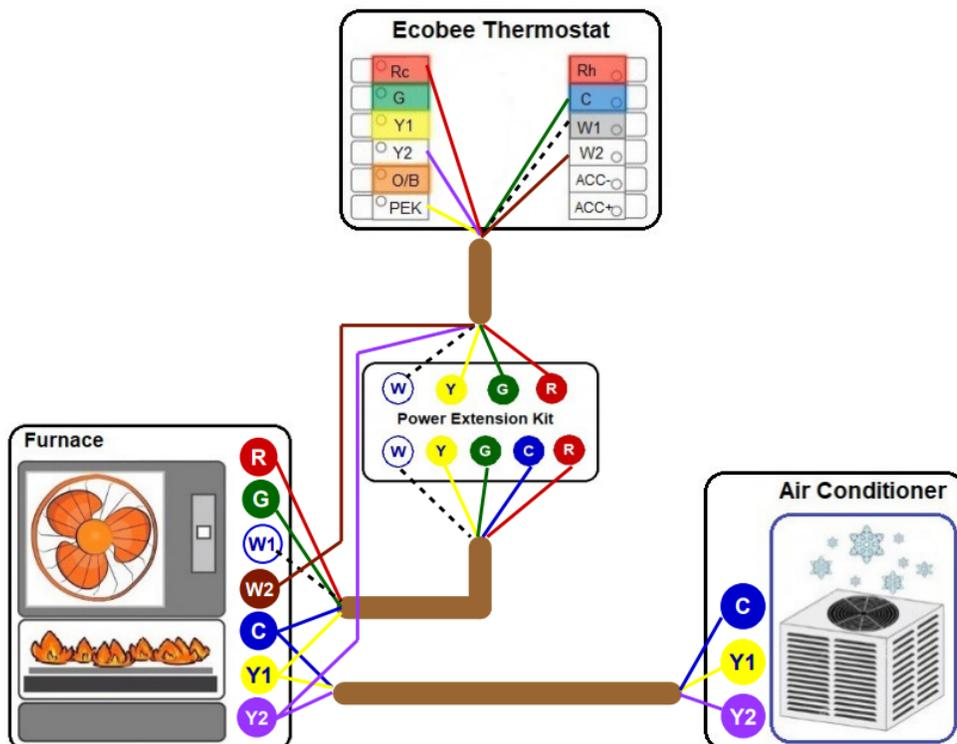
Diagram 5. Furnace (1-stage) + AC (1-stage)
