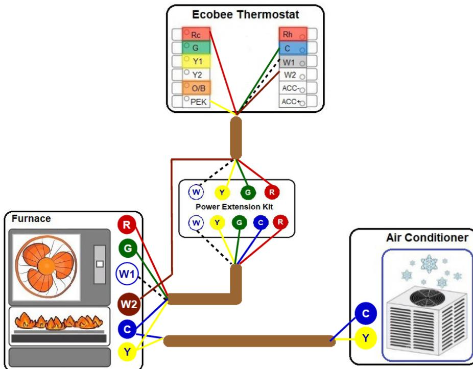
Diagram 3. Furnace (1-stage) + AC (2-stage) using PEK
