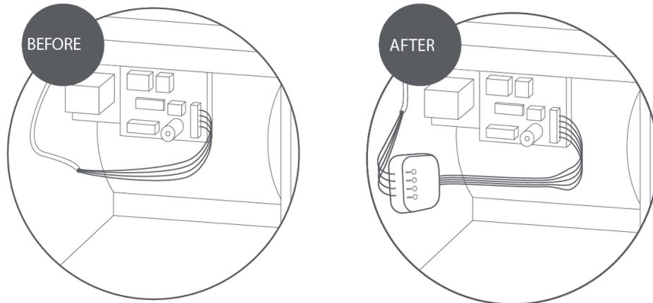
STEP 13: Mount the Power Extender Kit inside your HVAC system, taking care not to strain the wires. Close the HVAC cover panel securely and return to your thermostat.
