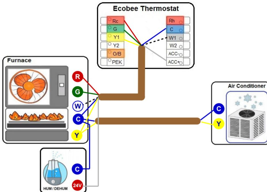
Diagram 21. How to Include a 2-wire Dehumidifier / Humidifier
