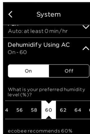
By enabling this threshold, your air conditioning system will overcool your home. It will stop once it reaches your overcool max setting or until the humidity set point is reached - **whichever occurs first**.
