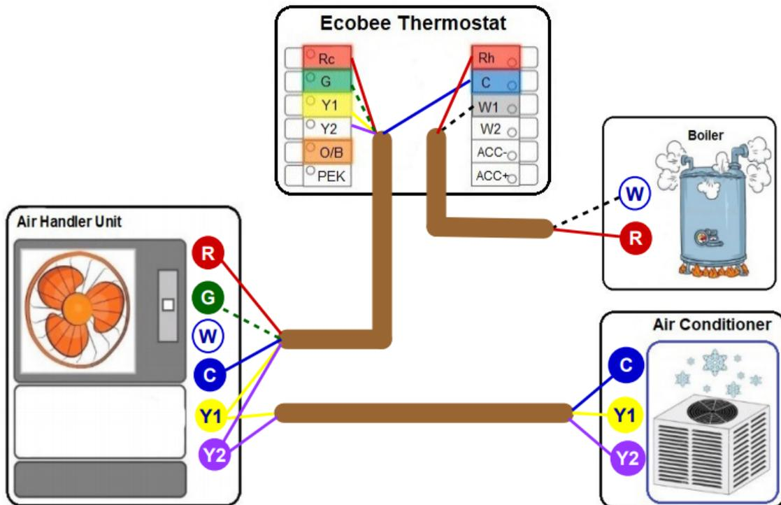
Diagram 25. Boiler (2-stage) + AC (2-stage) – 2 Transformers
