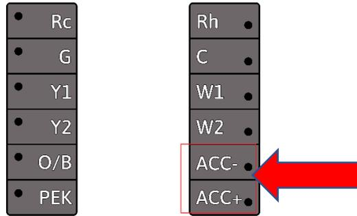
Once the ecobee has been wired to control the HVAC system and dehumidification system using the ACC+/ACC- terminals it will require correct setup to determine how you want to enable Dehumidification control. During the first-run setup they are a few key settings to ensure Dehumidification is part of the HVAC control algorithms.
