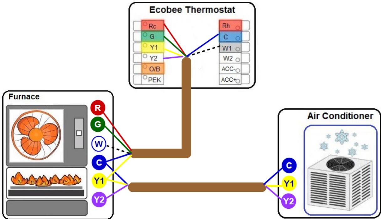
Diagram 8. Furnace (2-stage) + AC (2-stage)
