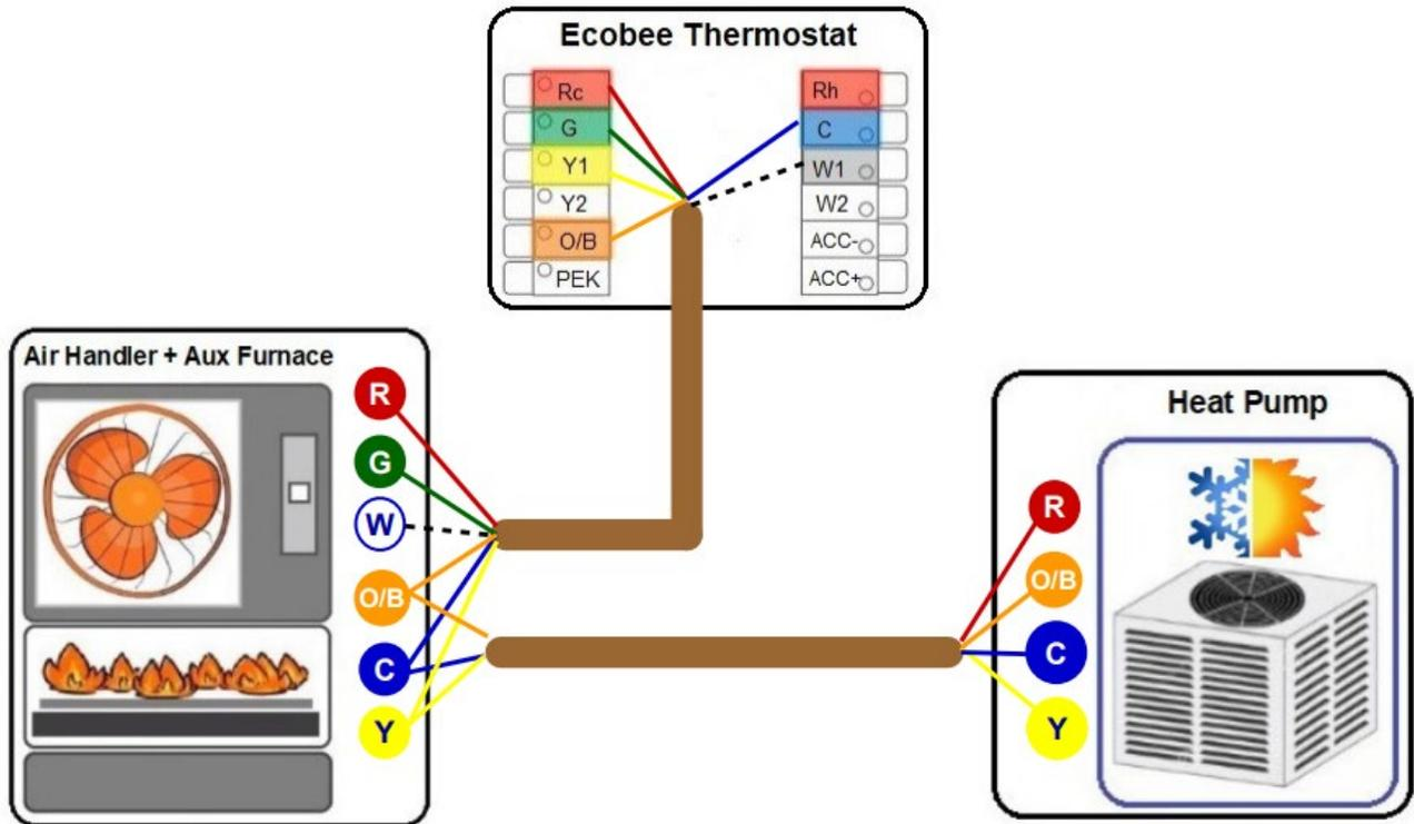
Diagram 14. Heatpump (2-stage) + Aux Heat (1-stage)
