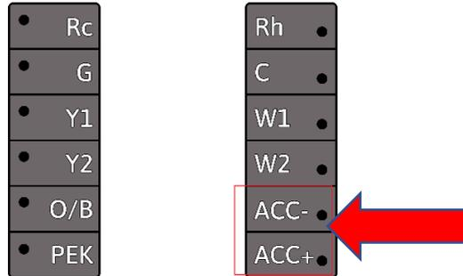
Once the ecobee has been wired to control the HVAC system and humidification system using the ACC+/ACC- terminals it will require correct setup to determine how you want to enable humidification control. During the first-run setup they are a few key settings to ensure humidification is part of the HVAC control algorithms.
