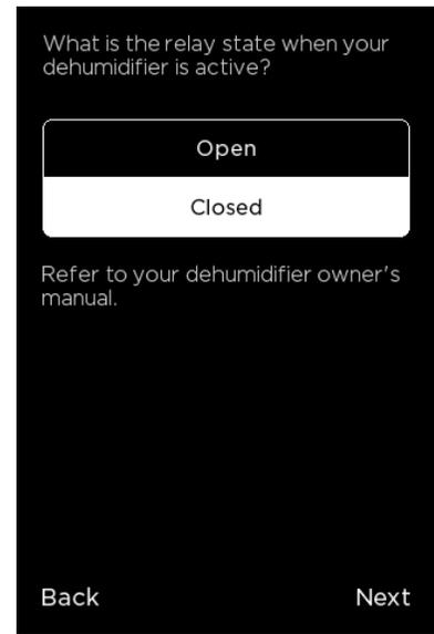
This setting determines if the state of the ACC+/- relay is **Open** or **Closed** when active. Refer to the HVAC equipment manual for the recommended setting.
