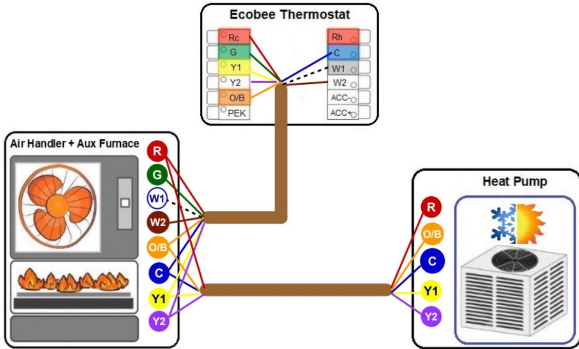
Diagram 16. Heatpump (1-stage) + Aux Heat (1-stage) using PEK
