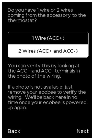
The ecobee will attempt to auto-detect the inserted wires into ACC+ / ACC-, therefore this prompt may not appear during setup.
