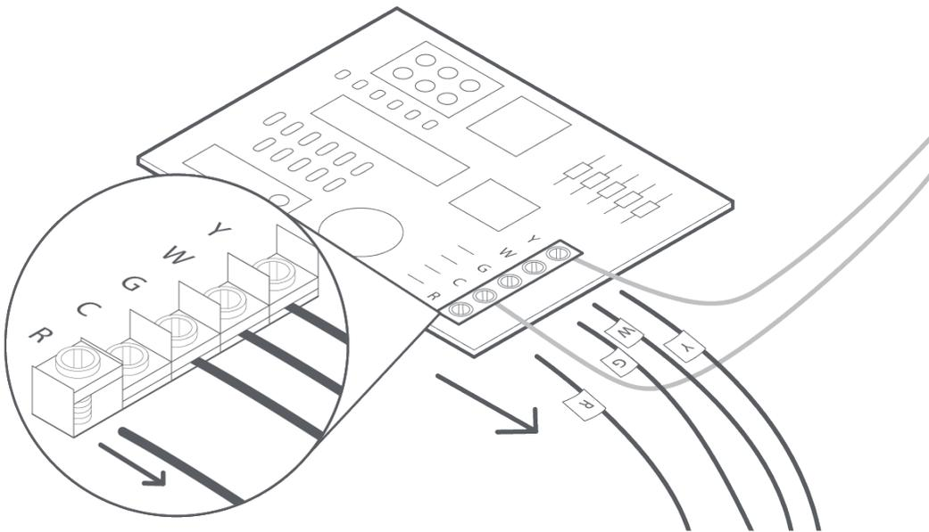
STEP 10: Connect the wires you disconnected from the control board into their matching gray terminal blocks on the Power Extender Kit.
