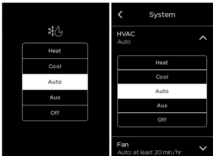
If the temperature goes above the blue cooling set point, the ecobee will turn on your cooling equipment to lower it down to the desired level. In the same way, the ecobee will turn on the heating equipment should the temperature drop below the heating set point.
