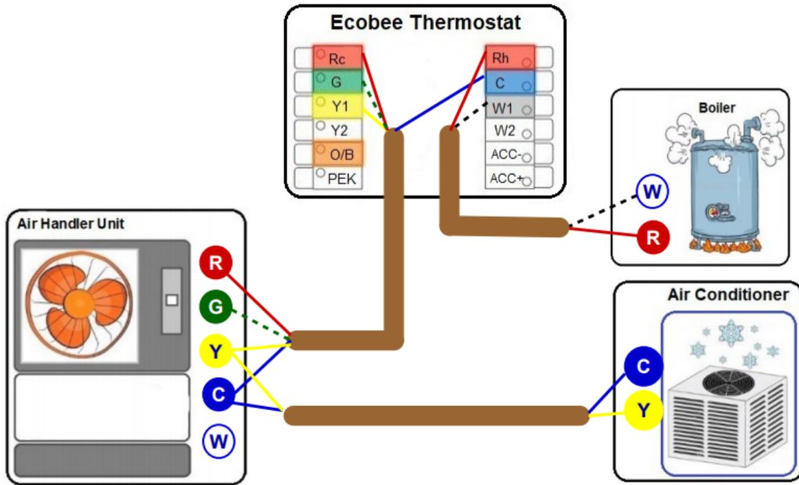
Diagram 24. Boiler (1-stage) + AC (2-stage) – 2 Transformers
