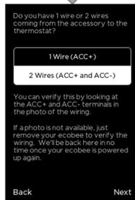
The ecobee attempts to detect if wires are inserted into ACC+/ACC- terminals and may not be prompted with the option.
