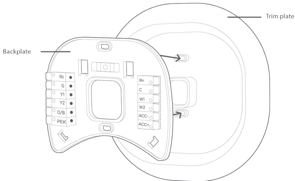
STEP 17: Pull the wires through the hole in the middle of the backplate and then attach the backplate to the wall using the drywall anchors and screws provided.
