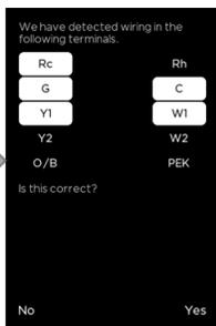
The ecobee attempts to detect the wires inserted in the backplate terminals. If a wire has not been detected, you can tap on "No" to modify
