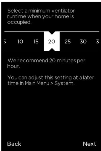
**Ventilator Minimum On Time While Home:** The number of minutes per hour the fan is required to run when the house is considered occupied
