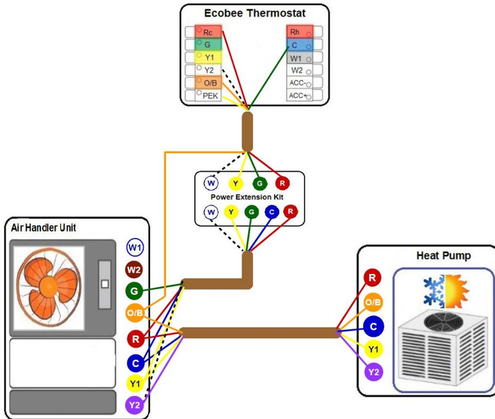
Diagram 13. Heatpump (1-stage) + Aux Heat (1-stage)
