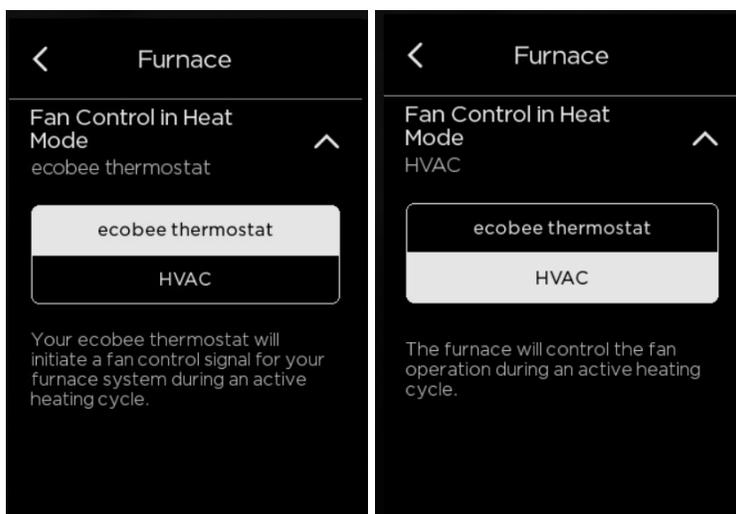
Set to **ecobee thermostat**: By choosing this option, your ecobee will energize the fan directly during heating cycles. This will cause the fan to immediately turn on when a heating cycle is initiated and continue to run until the heating cycle ends.
