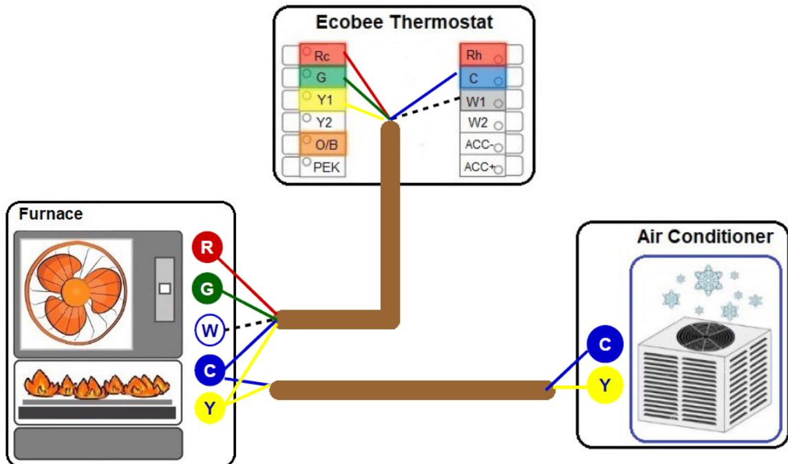
Diagram 6. Furnace (2-stage) + AC (1-stage)
