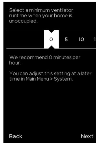
**Ventilator Minimum On Time While Away:** The number of minutes per hour the fan is required to run when the house is considered unoccupied
