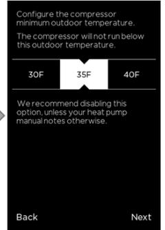
Typical of an air-to-air heatpump system, as outdoor air becomes cooler the Heatpump will become less effective. This setting determines when the heatpump is turned off and switches to auxiliary heat. Refer to your HVAC equipment manual for your optimum setting.
