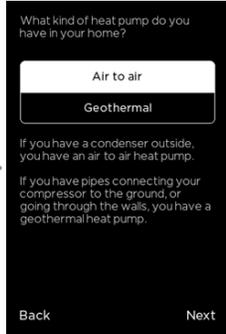
Air to air Heatpump systems are most common. If the condenser is located outside this is a typical air-sourced heatpump.
