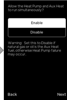
This setting will allow the Heatpump and Aux Heating to run simultaneously. It is very important that the heatpump evaporator coil is physically installed upstream of the Aux Heating source. Otherwise, heatpump failure may occur.
