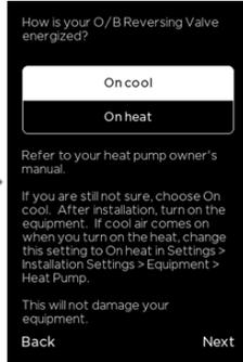
The O/B Reversing valve requires configuration based on the default mode of your heatpump. Engage R/V "On cool" is more common.
