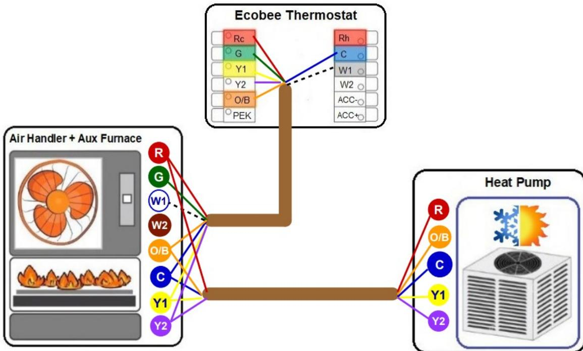
Diagram 15. Heatpump (2-stage) + Aux Heat (2-stage)
