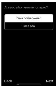
Only select "I'm a pro" to access the multi-speed fan options for 2-pipe/4-pipe fan coils or PTAC's. Otherwise leave the default setting.
