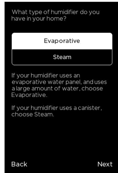
This setting determines the type of humidifier system. Evaporative is recommended to operate with a heating cycle.
