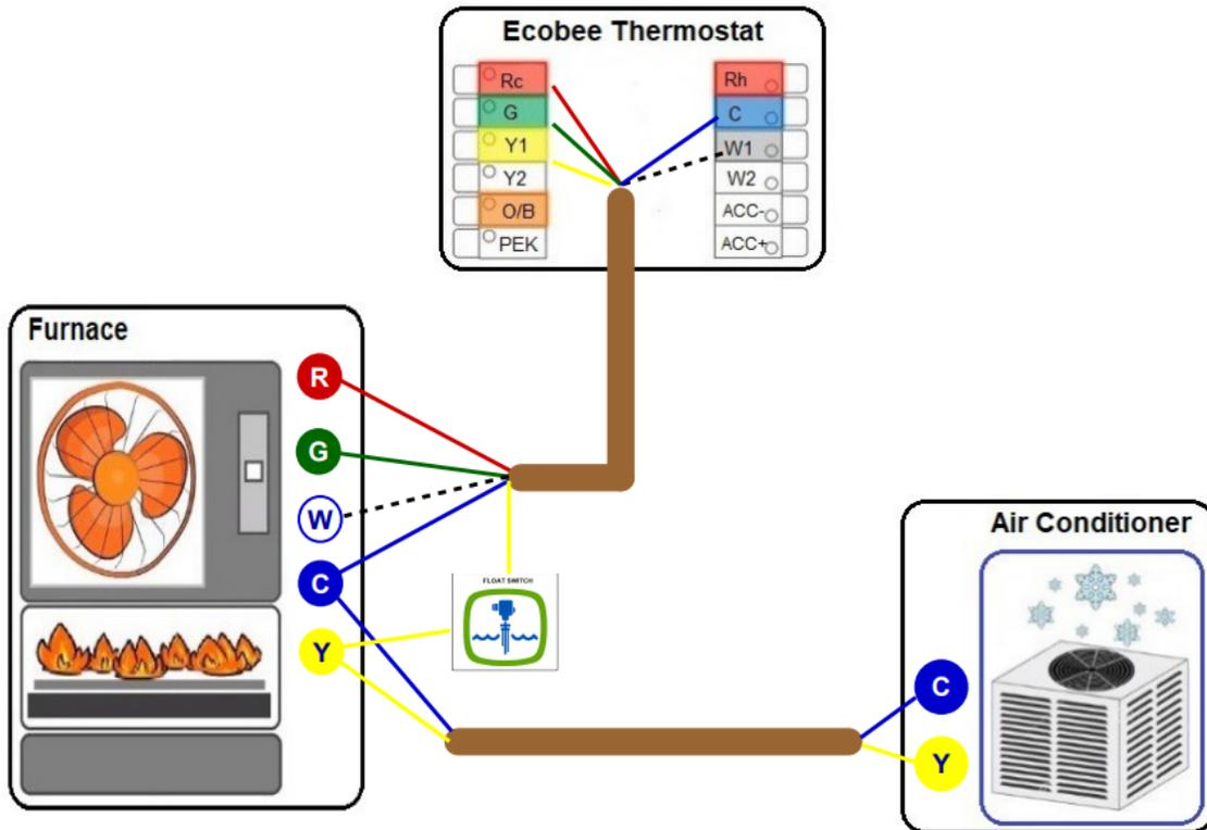
A float switch will prevent the AC from running if the drain pan is full of water or condensation pump motor fails.
