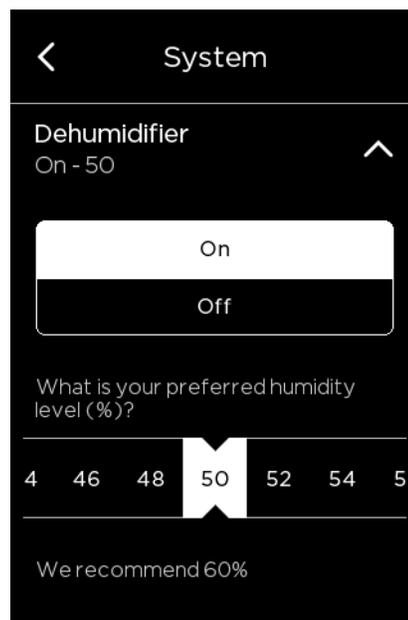
AC Overcool Max is another option to help control high humidity levels and works in conjunction with the Dehumidify setpoint under System Mode menu. This setting will allow the Air Conditioner to overcool by comparing the actual RH% vs. the desired Dehumidify setpoint.
