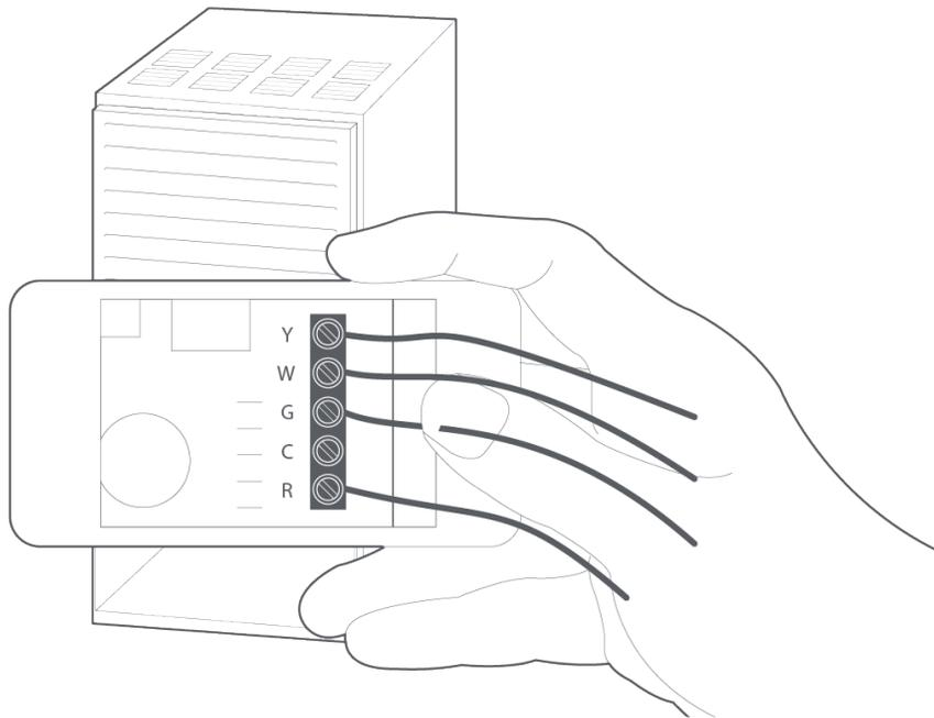
STEP 8: Label only the R, Y or Y1, G, and W or W1 wires with the matching labels provided. If you have more than one wire going into these terminals, only label those going to your thermostat.
