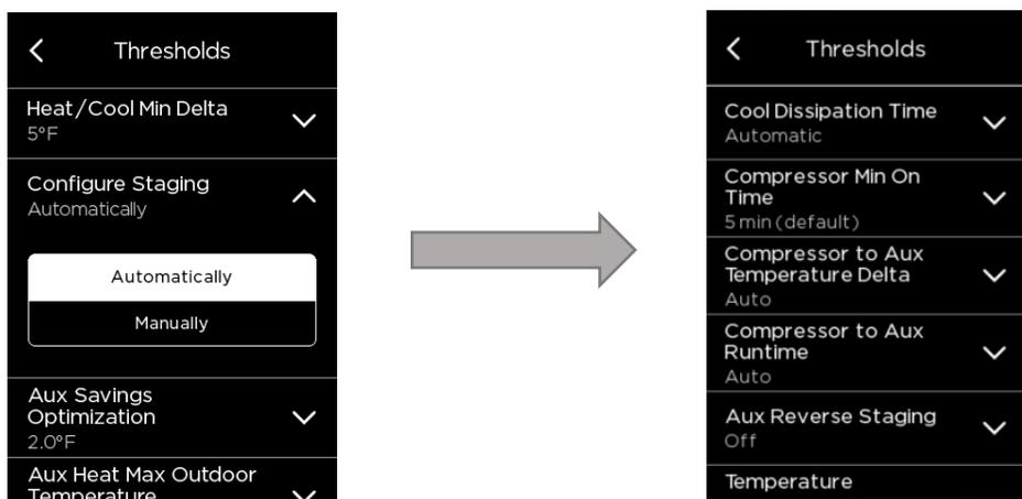
For heat pump systems, its also crucial to understand what the minimum outdoor temperature that the heat pump can run with - otherwise the thermostat will lock out the heat pump and change over to aux heat as the weather outside will be too cold to run the heat pump unit that is sitting outside.
