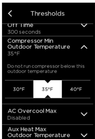
To also avoid short cycling and increase equipment efficiency, you can go to **MENU → SETTINGS → INSTALLATION SETTINGS → THRESHOLDS → HEAT DIFFERENTIAL TEMP →** and change this to a higher value so that the system turns on for a larger temperature drop and reduces short cycling.
