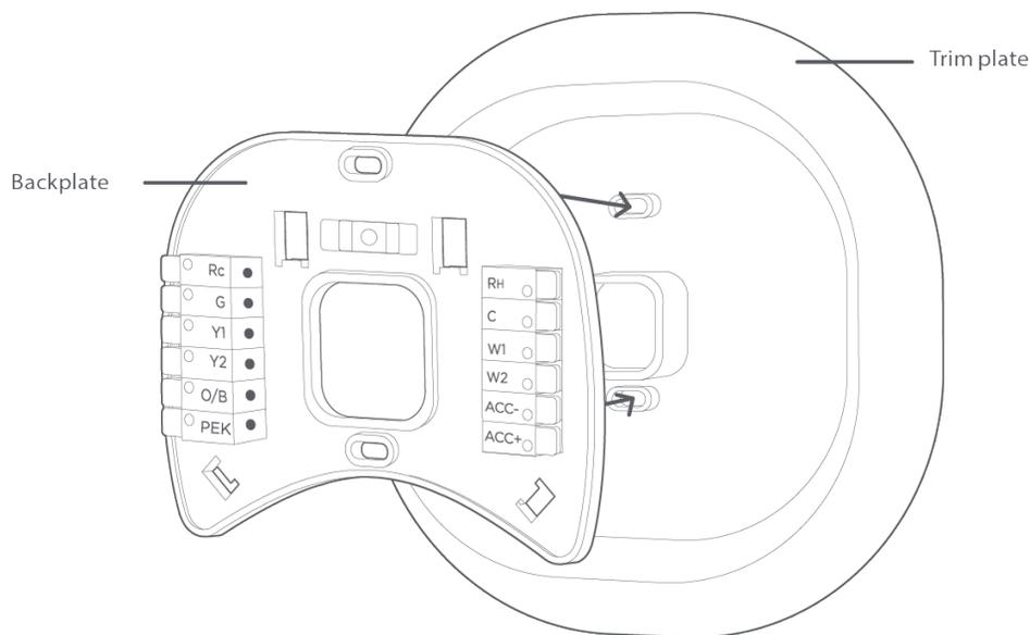
STEP 8: Pull the wires through the hole in the middle of the backplate and then attach the backplate to the wall using the drywall anchors and screws provided.
