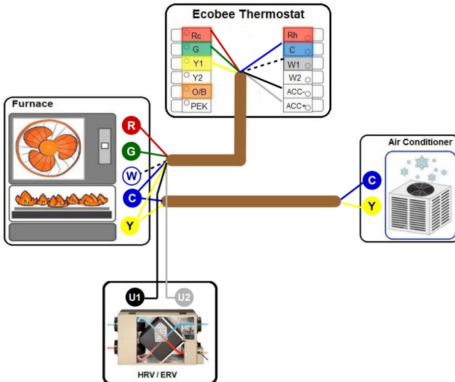
Diagram 23. Boiler (1-stage) + AC (1-stage) – 2 Transformers
