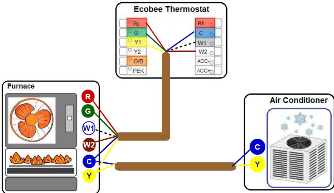
Diagram 7. Furnace (1-stage) + AC (2-stage)
