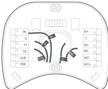
STEP 9: Insert your remaining wires into the side (not the front) of their corresponding terminal blocks.
