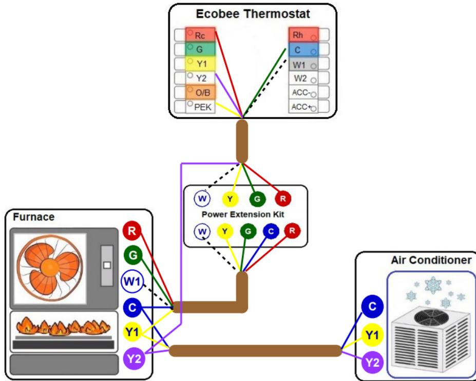
Diagram 4. Furnace (2-stage) + AC (2-stage) using PEK
