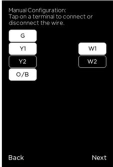
When O/B is configured with any combination of other wires this is defined as a heatpump system.
