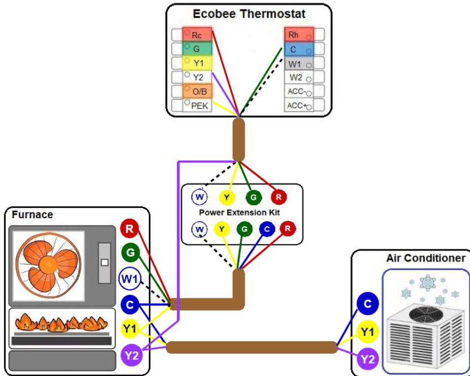
Diagram 18. Heatpump (2-stage) + Aux Heat (2-stage) using PEK
