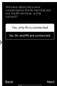
"Rc only" indicates the HVAC system has a single 24V transformer. When "Rc/Rh" is selected a typical dual 24V transformer system is a separate heating boiler with a separate forced-air AC system. Do not modify unless you have the latter of the two options.
