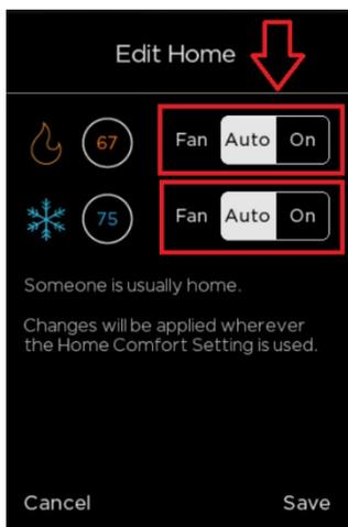
The ecobee has two modes of fan operation: **Auto** and **On**
