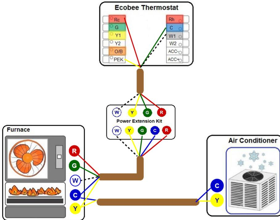
Diagram 2. Furnace (2-stage) + AC (1-stage) using PEK
