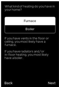
This setting determines the heating system type. Furnace refers to forced-air heating systems that have ductwork with floor/wall vents. If the system is hot water/hydronic heating select Boiler, otherwise leave the default setting to Furnace.
