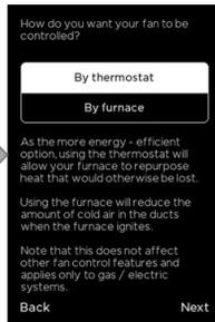
Using the default "By thermostat" setting provides user selectable heat & cool fan dissipations to help maximize residual heat or cool from the HVAC system.
