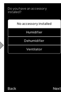
Ecobee3, ecobee4 & Smart Thermostat w/voice support an Accessory terminal. If no Accessory is connected, leave this setting at the default setting.
