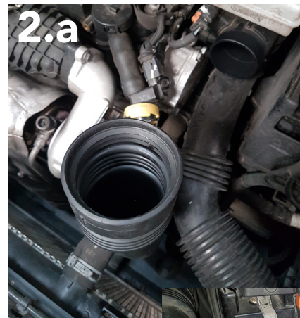
Air filter line inlet
