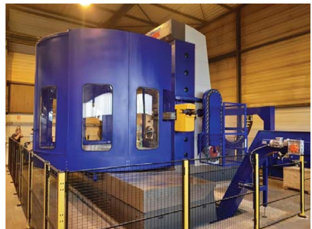
TOS 7 Axes CNC horizontal boring Machine at our STRAHMAN MGS plant in Vaux Sous Aubigny, France.
