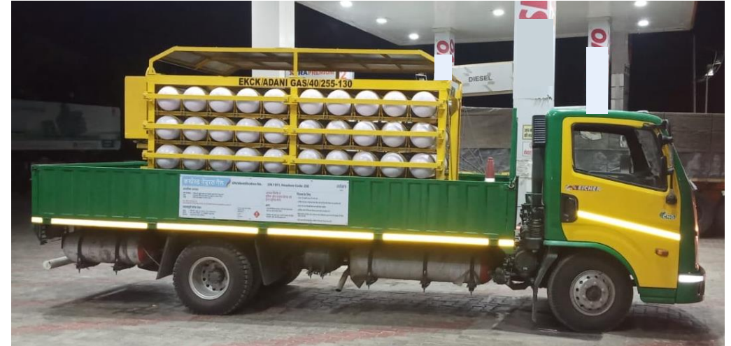
CNG run Cascade LCV already in use
