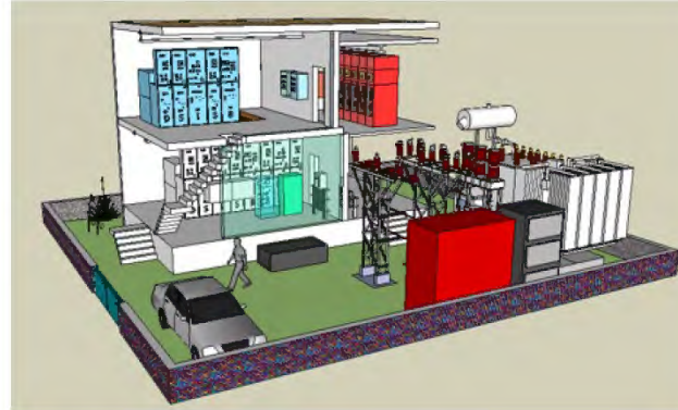
Compact 33 kV Distribution Station
