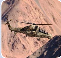
Light Combat Helicopter (LCH) - Capable to operate at 4700 mtrs with a payload of 500 kg
