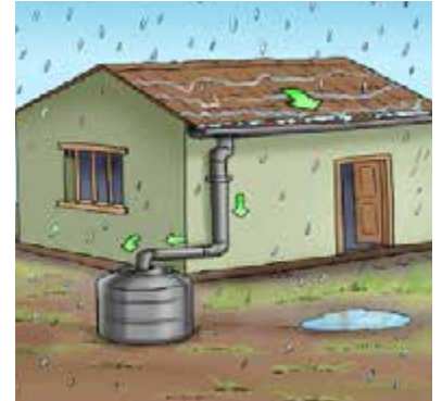
Rain Water Harvesting and other storage units
