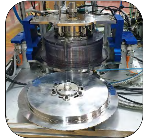
In-house developed sub-assembly for double-capsule filter manufacturing
