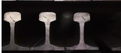
Head hardened grade 1080 HH rails for critical railway application
