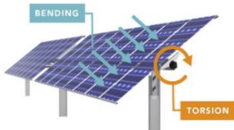
Transmission Shaft Tubes in Solar Tracker Structure (Magsure – Coated)
