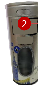
0.15mm DR08 Tinplate 5.6/5.6 coating, Heat Reflector (Replacing Alumnized Steel)
