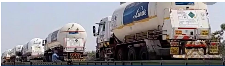
Road Tankers being moved by Railway (Roll-on, Roll-off)
