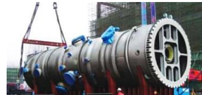
Coal Gasifier for China
