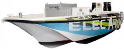
Country's maiden fuel cell technology vessel with zero CO<sub>2</sub>, NO<sub>x</sub>, SO<sub>x</sub> emission and cost effective sustainable green energy solution for inland waterways application. Proof of concept is already completed, 24 pax vessel is under development.
