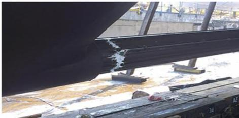
Minimization of launch induced deflection by installation of technical shaft to simulate the solid reference axis (Pre-alignment condition) for facilitating completion of structural shafting job on slipway before launching.
