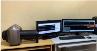
R&D initiatives in association with Academia and start-up - developed as the replacement of film X-ray technique that is used currently in conventional radiography for weld inspection
