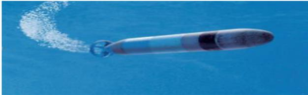
b) Mobile Target Emulator (MTE): Attracts the torpedoes away from the counter maneuvering Submarine (target) by emulating the acoustic and dynamic behavior of a target submarine.
