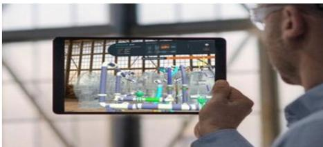
Providing 3D CAD model pulled from Design on hand held devices like iPads and 3D Goggles (HoloLens) superimposing on compartments physical structural boundaries resulting in reducing re-work and reduction of valuable project completion time and cost.
